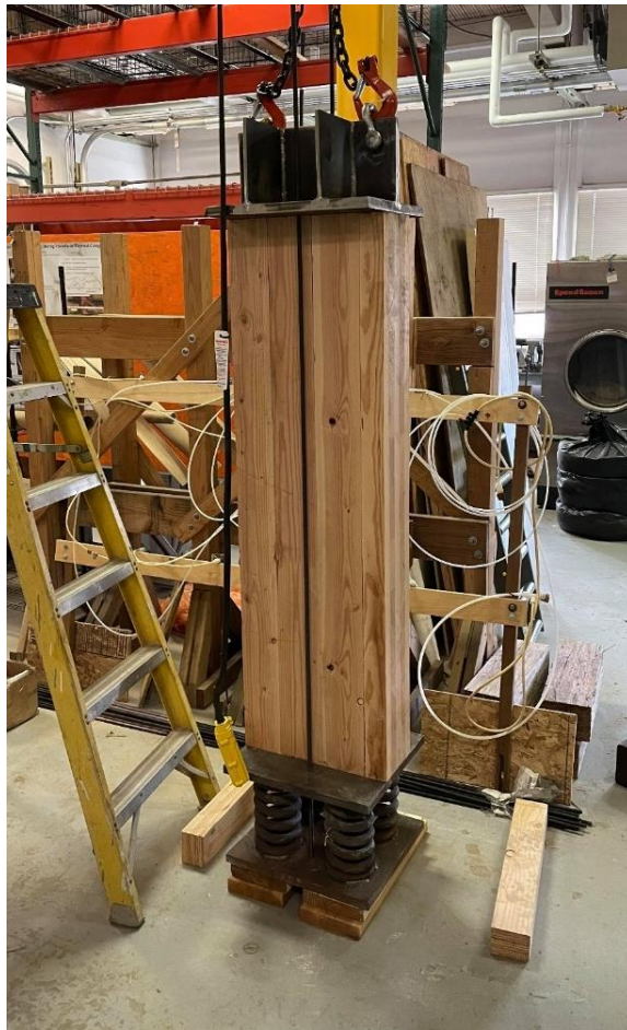
Figure 4.5. Small-scale CLT specimen attached to a crane as a safety precaution.
