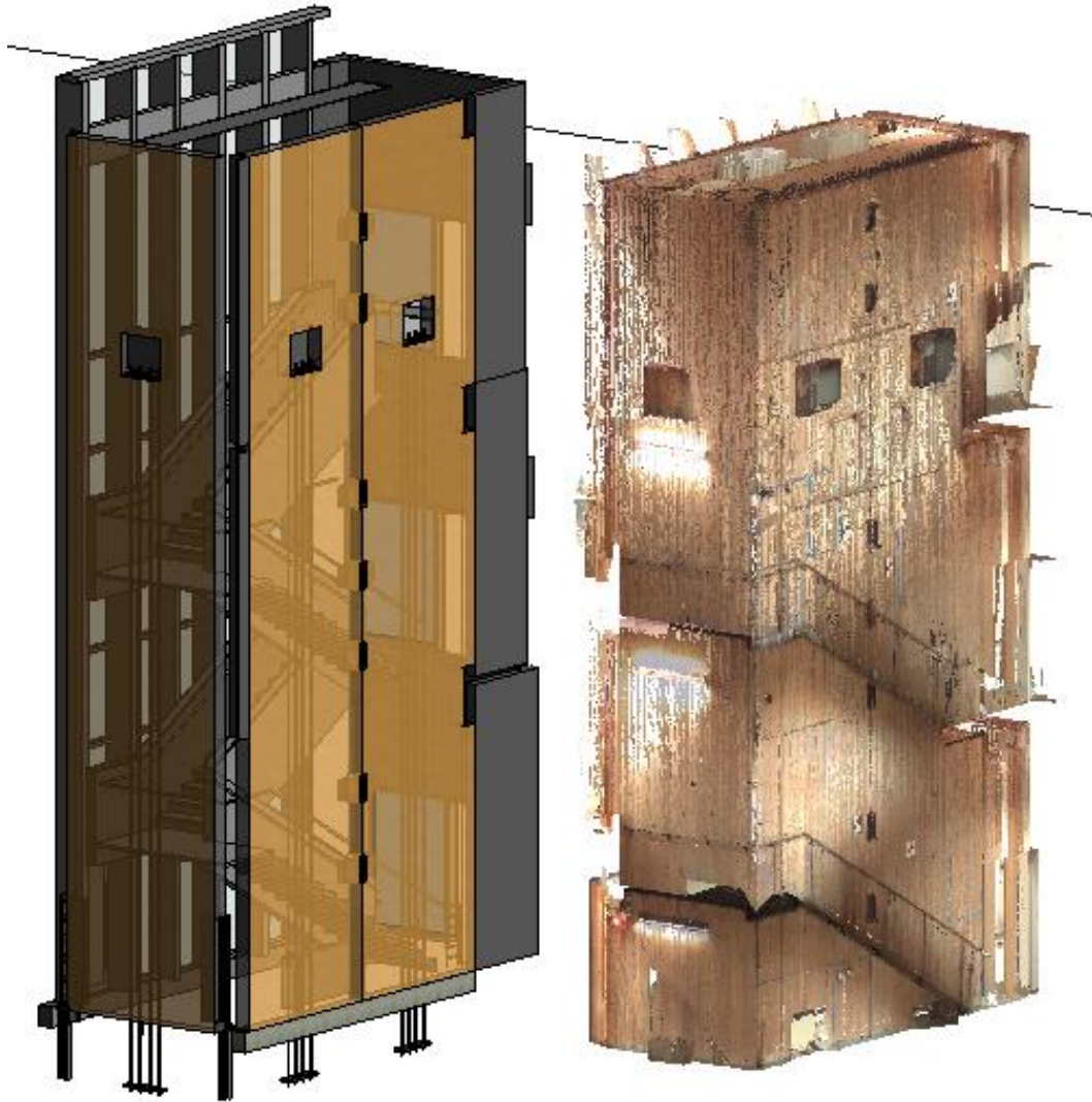
Figure 5.3. Building Information Model (left) and point cloud model (right)
