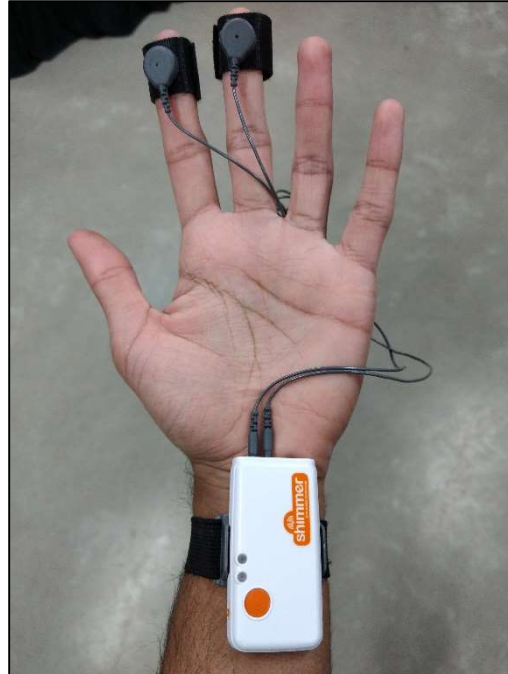
Figure 3.1: Shimmer GSR+ sensors (shown attached to the index and middle finger) send data to a host computer through the wireless transmitter (shown attached to the wrist) in real time
