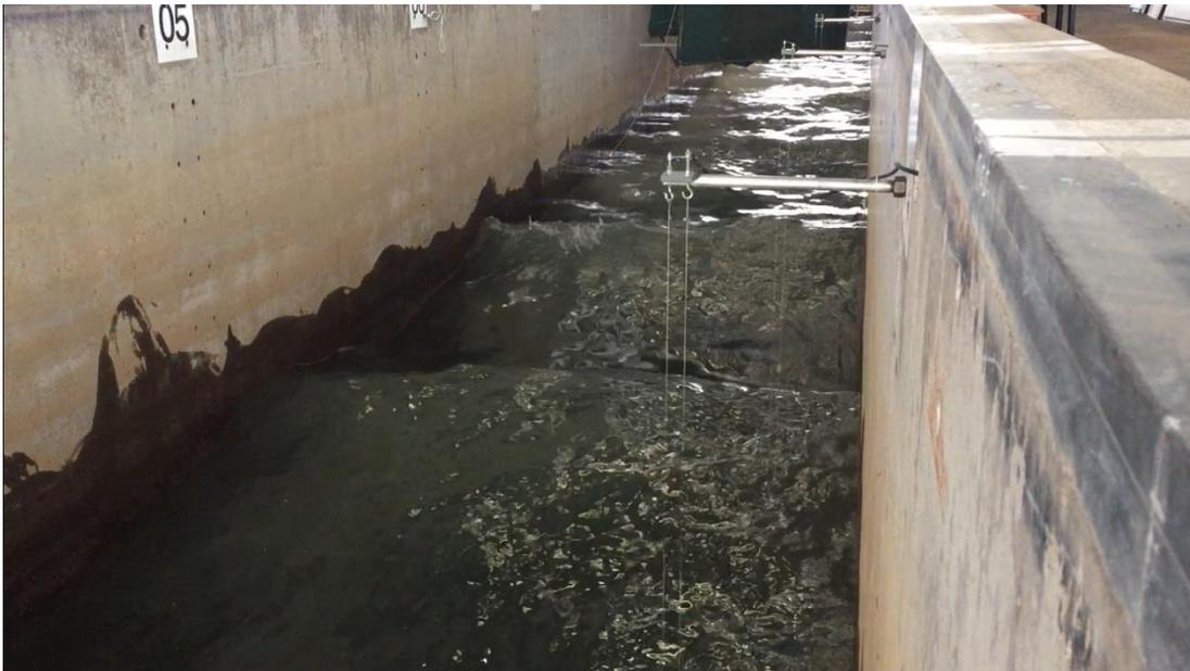
Figure 4.4: Resistance wave gauge 2 during testing.
