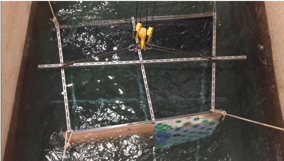
Figure 4.7: Wave damper during deployment.
