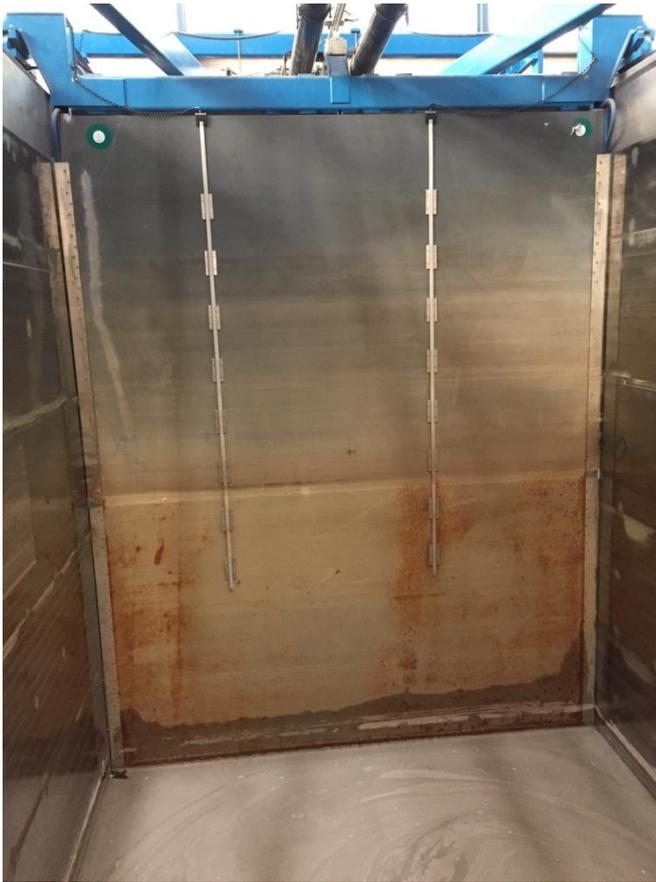
Figure 4.6: Wavemaker wave gauges (wmwg).
