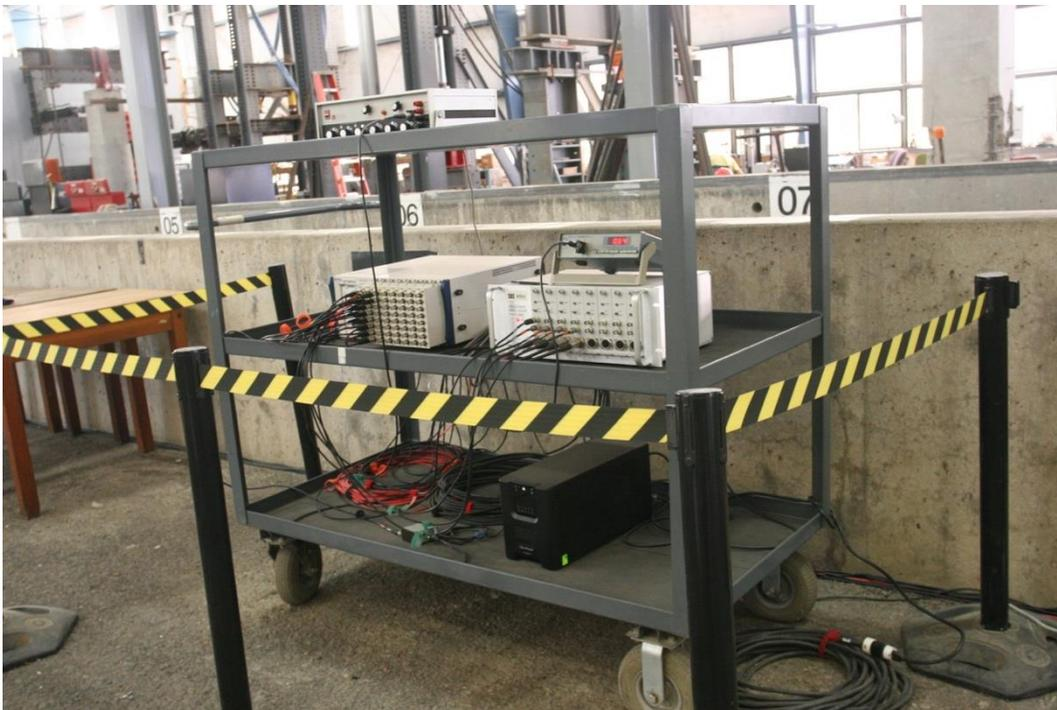
Figure 5.1: ImTech resistance wave gauge, voltage standard, and DAQ.
