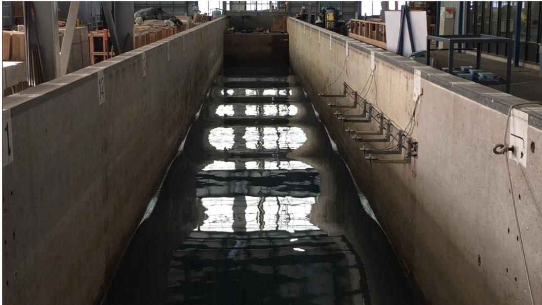
Figure 4.5: Acoustic wave gauges 1-8 shown during testing.
