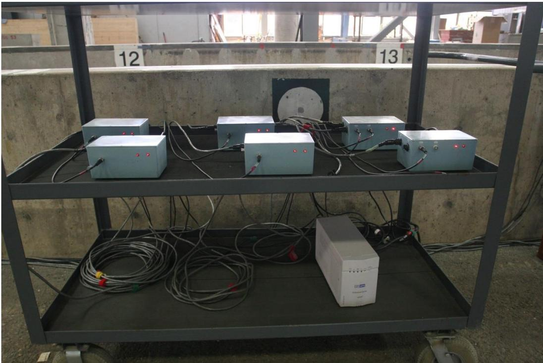
Figure 5.2: System setup used to send the ultrasonic wave gauge measurements to the data acquisition system.
