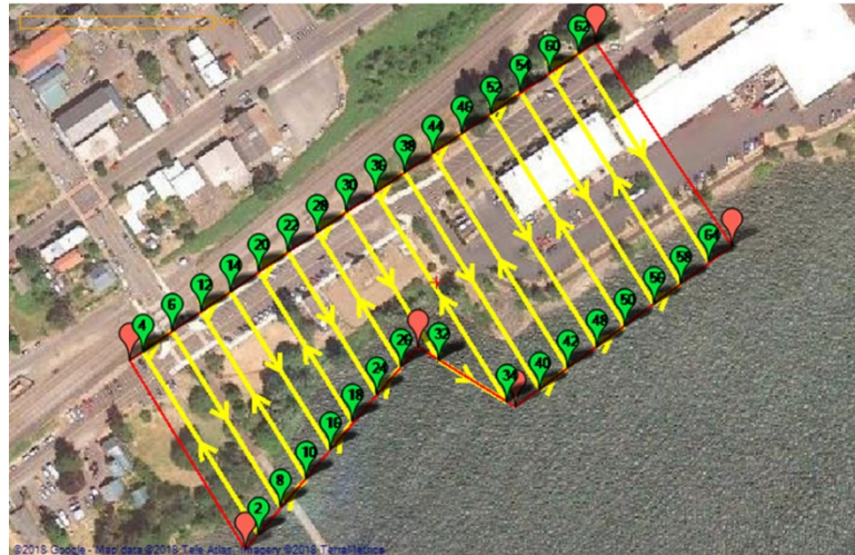
Figure 11: The waypoint mission plan used to acquire the aerial imagery as created by ArduPilot's Mission Planner software.
