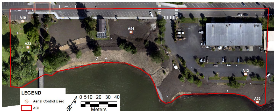
Figure 14: The five control points used for the the SfM processing. For datasets where only one control point was used the aerial target located nearest to the center of the AOI was used; Point ID A54. For the datasets utilizing 5 control points the aerial targets located nearest to the four corners of the AOI, and the center point was used; A12, A19, A23, A52, and A54
