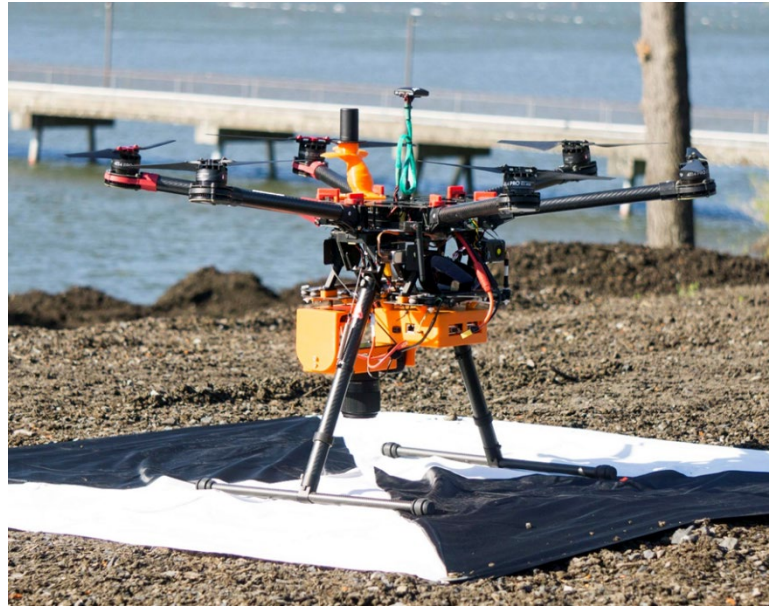
Figure 10: The s900 airframe with Piksi Multi GNSS Receiver, GNSS antenna, and Sony A6300 camera with sigma 30mm lens prior to takeoff.
