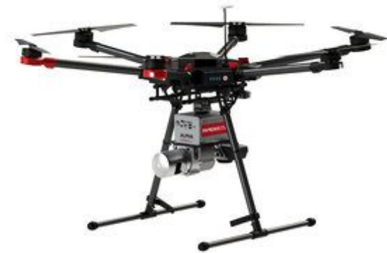
Figure 15: The Phoenix Aerial al3-32 Scanner mounted on a DJI m600 Pro. Image courtesy of Phoenix Lidar Systems, https://www.phoenixlidar.com/al3-32/
