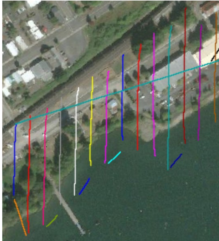
Figure 16: An image of the 20 flight lights used for acquiring the aerial lidar dataset.
