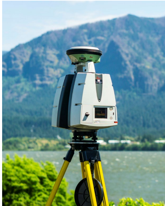
Figure 6: The Leica P40 Lidar scanner with a Leica GS14 GNSS antenna mounted on its top during one of the 10 scan position observations.
