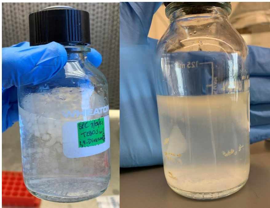
Figure 4.2. Images of the T2BOS 1 gellan gum bead batch reactor taken at the start of the study (left) and taken 47 days into the study (right).
