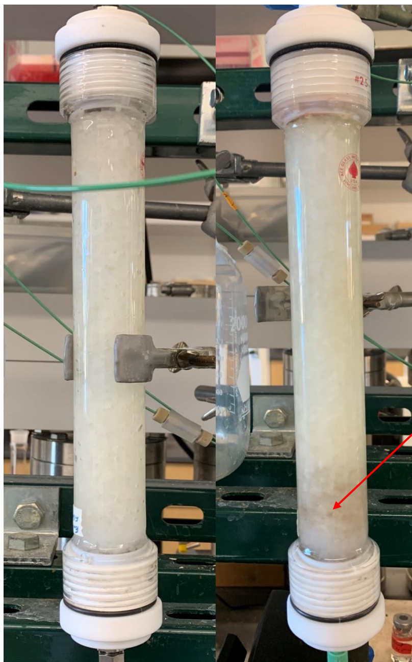
Figure 5.8. Images of the T2BOS gellan gum bead column from the start of operation (left: 0 PV) and the end of operation (right: 117 PV). The red arrow indicates the darkened area that became more prevalent over time.
