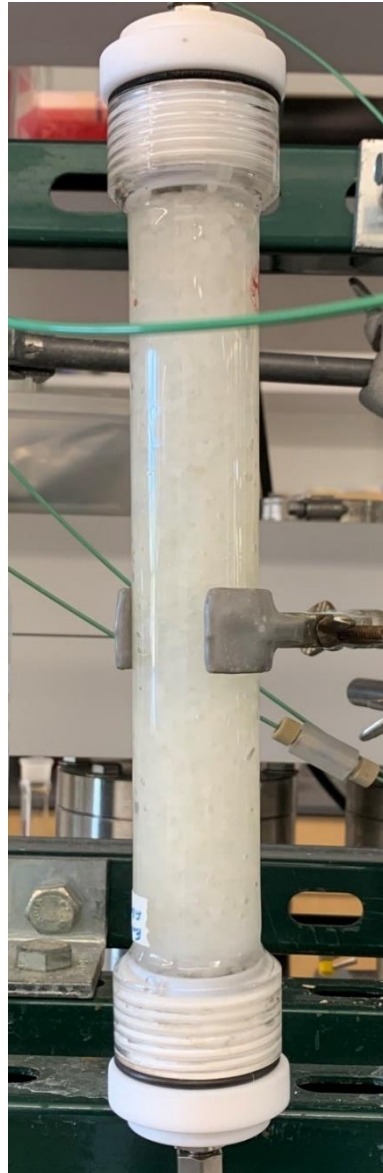
Figure 5.1. Image of the T2BOS gellan gum bead column taken at the start of its operation.
