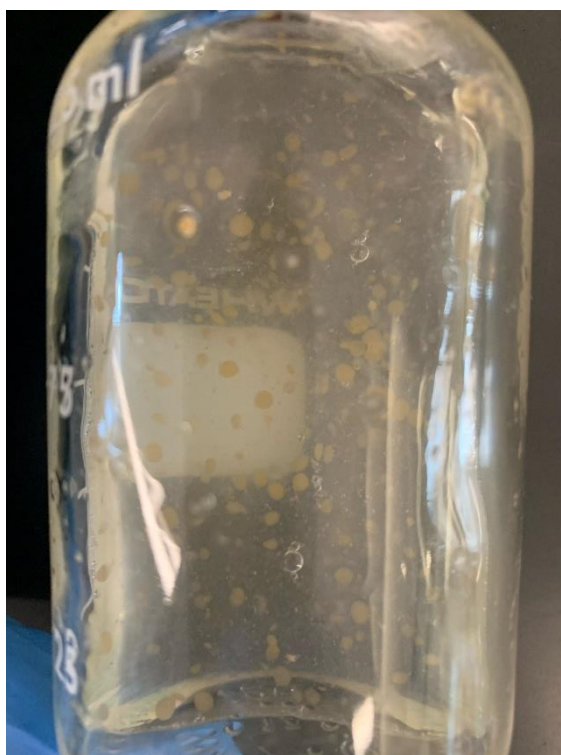
Figure 4.5. Image of the TBOS 1 gellan gum bead batch reactor taken at the end of the batch bottle study.
