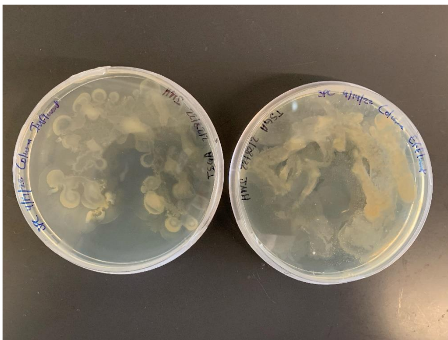
Figure A.3. Pictures of streak plating onto TSGA plates of liquid taken from the column influent section (left) and the column effluent section (right).
