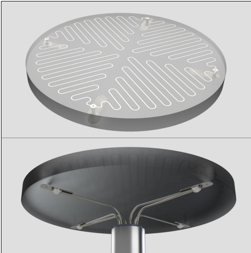
Figure 4-12: CAD model render of the proposed HERTEL sensor, top and bottom faces
