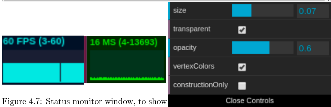
Figure 4.8: Control panel to make visualization status change, including opacity, point size, color shader and construction points filter.
