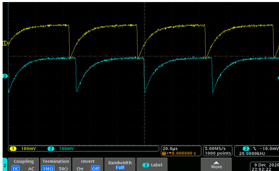
Fig. 60. Signal from the two channels that was fed to the DPP8 for coincidence testing
