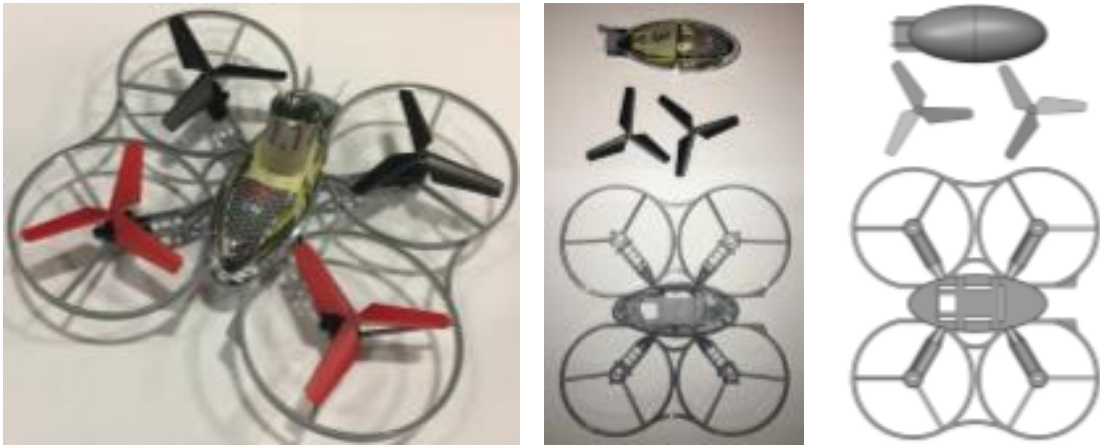
Figure 9. Testing with various weights (left), disassembled quadcopter (middle), and CAD models (right)
