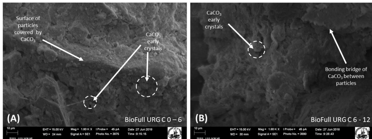
Figure 7 - BioFull on URG C at three different sample depths (A, B, and C). All images are under 1800 X TM
