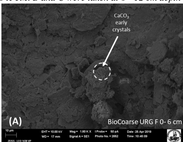
Figure 2 - BioCoarse on URG F at two different sample depths. Image A and C are under 1800 XTM, and B is under 250 X TM. B and C were taken at 6 - 12 cm depth in the sample.
