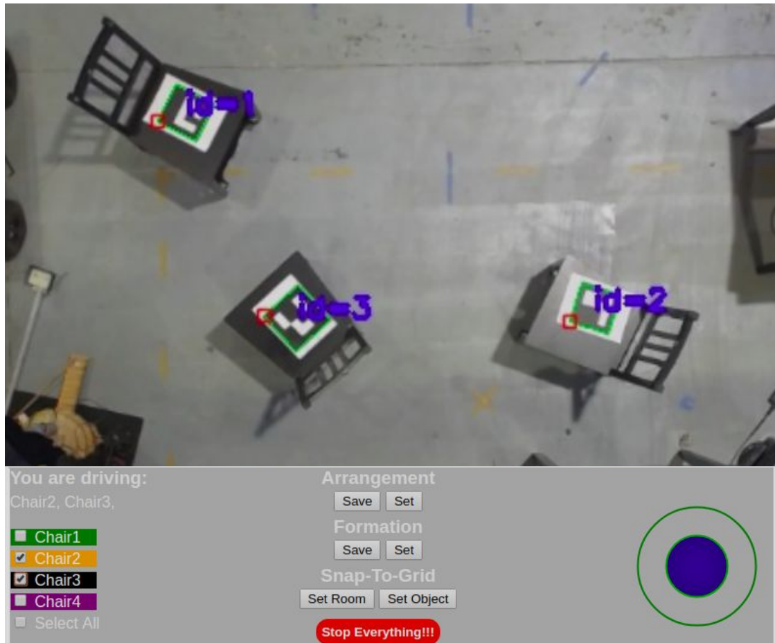
Figure 4.6: Screenshot of the ultimate screen-based user interface. It consists of a live video stream of the room, and affordances for controlling the ChairBots. Affordances include a ChairBot selector, autonomous capabilities to set and save both arrangements and formations, and an option to snap to an orientation as well as low-level motion (with the joystick) and emergency stop controls. A demo video is available at [65] .
