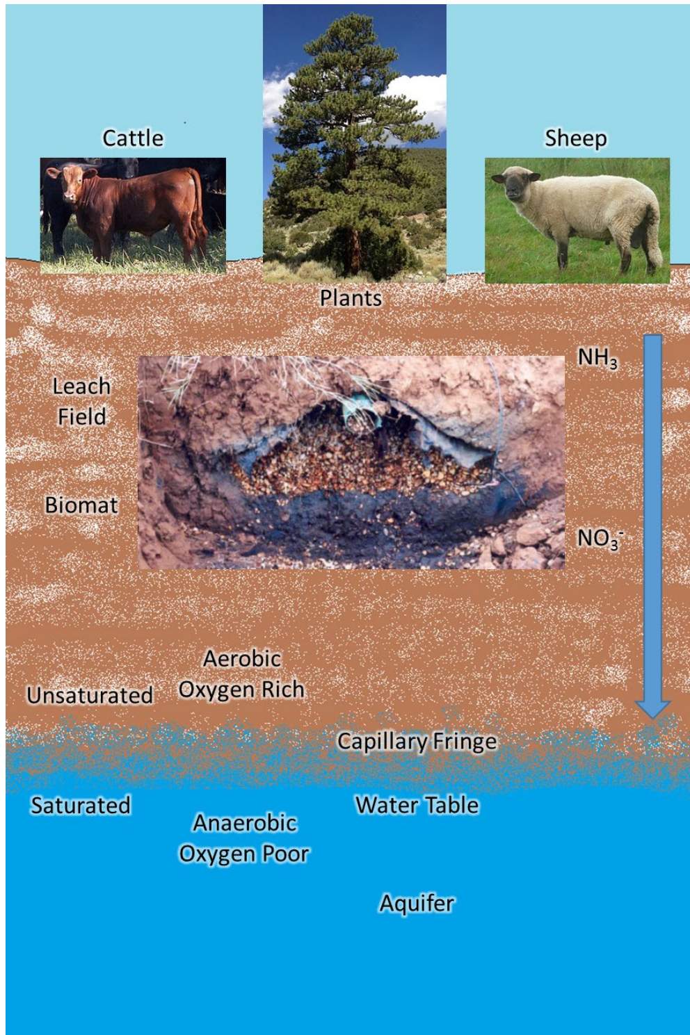
Fig. A2. Nitrogen Transport and the Subsurface Leach Field image from (Rainwater and Jackson, 2004); other images are open source.
