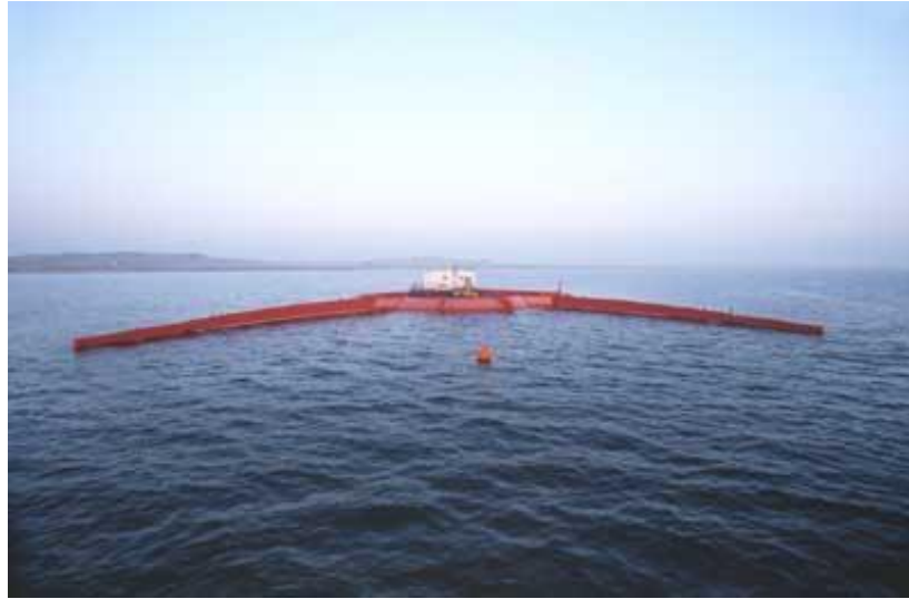
Figure 2: The world's first offshore wave energy converter, the Wave Dragon, is an overtopping device.
