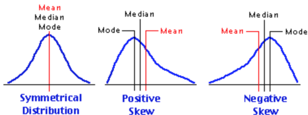
Figure 4: Skewness can be indicated by the difference of the median (50th percentile) and the mean. Larger differences between percentiles and the mean determine the degree to which the distribution is skewed. (CFA, 2020)
