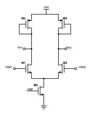
Fig. 3.27 Preamplifier in the comparator
