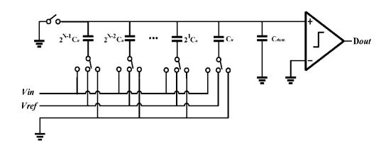
Fig. 2.2 SAR ADC with binary weighted DAC
