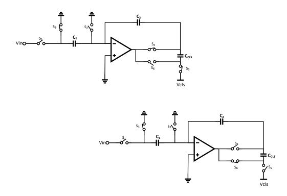
Fig. 3.17 Two operation phases of CLS
