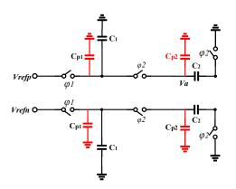
Fig. 3.18 Mismatch and parasitics in 2-C DAC
