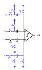
Fig. 3.26 Passive adder for calibration
