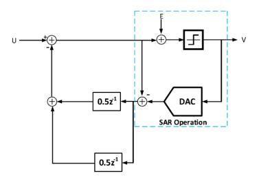
Fig. 2.6 First order NS SAR in fully passive [3]
