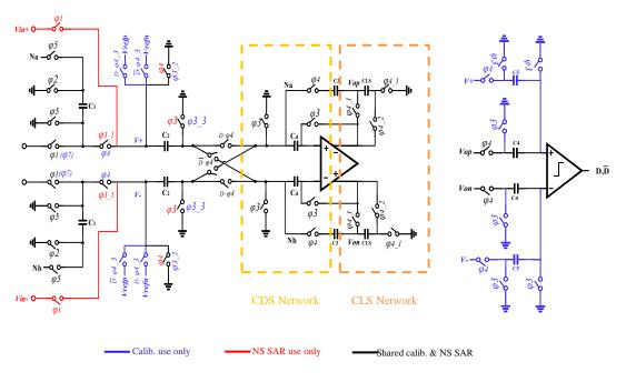
Fig. 3.4 Block diagram of proposed ADC
