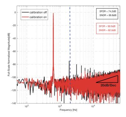
Fig. 3.31 Measured PSD of proposed ADC
