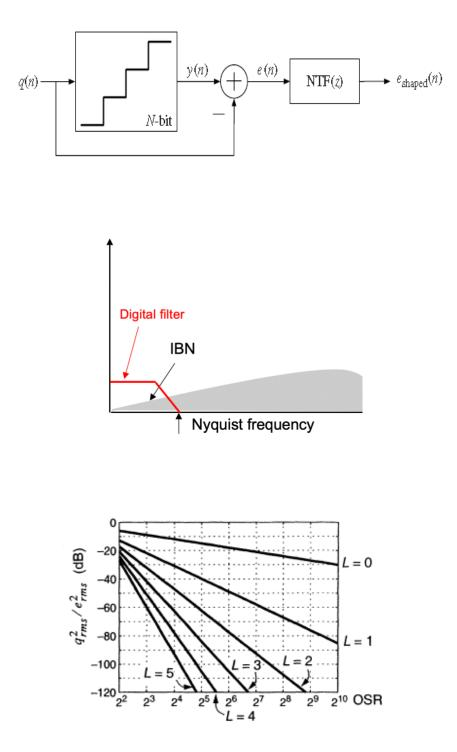
Fig. 2.5 (a) Concept of noise-shaping, (b) noise distribution with noise shaping, (c) noise attenuation versus OSR and order of noise shaping
