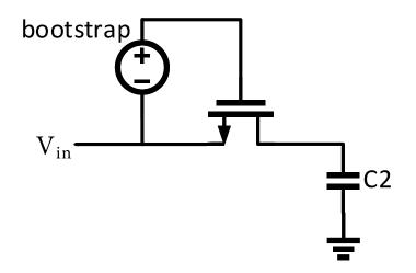
Fig. 2.16 Simplified bootstrapped switch
