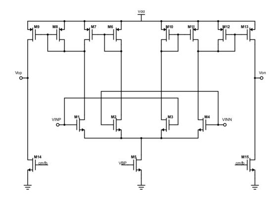
Fig. 3.24 Current mirror integrator op-amp
