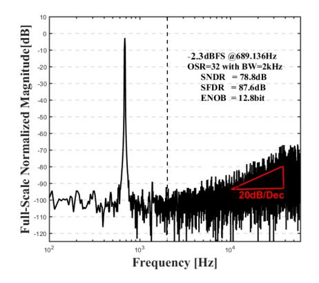
Fig. 2.19 Measured PSD
