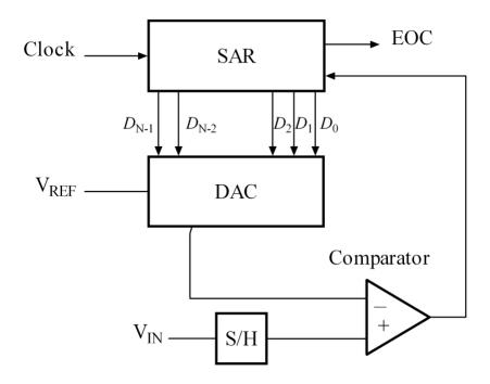
Fig. 2.1 Conceptual block diagram of SAR ADC
