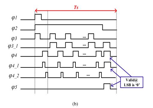
Fig. 3.5 (a) NS SAR conversion mode configuration, (b) Timing diagram
