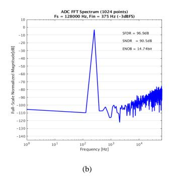
Fig. 3.16 CDS noise simulation (a) CDS only works in sampling phase, (b) work in each bit conversion
