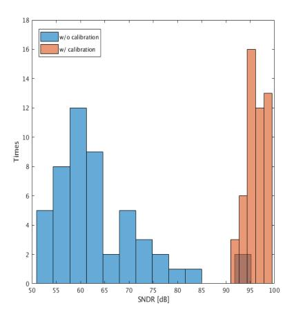
Fig. 3.19 Monte Carlo simulation of DAC mismatch
