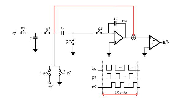
Fig. 3.21 First step of calibration
