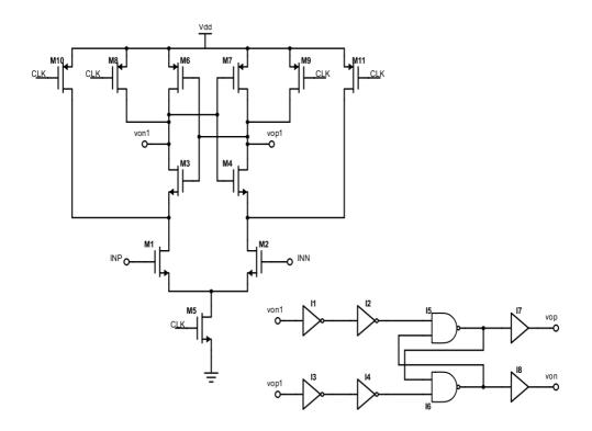
Fig. 3.28 Latch used in comparator
