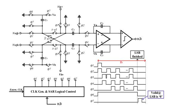
Fig. 2.8 Proposed NS SAR ADC architecture and operation timing
