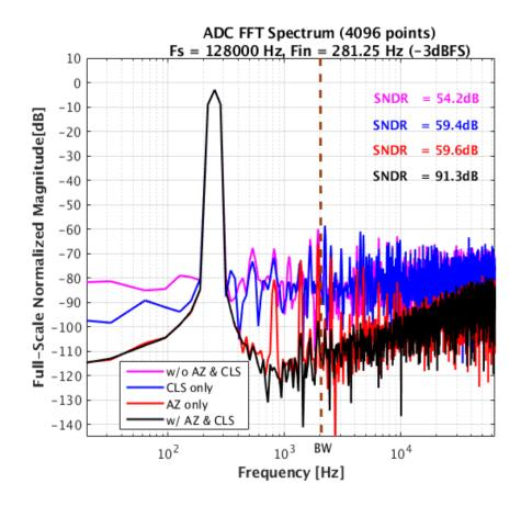
Fig. 3.14 Performance comparison w/ and w/o CDS and CLS
