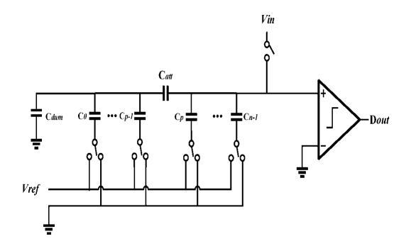
Fig. 2.3 SAR ADC with binary weighted DAC w/ attenuation cap
