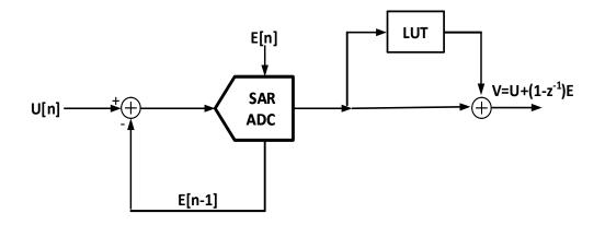
Fig. 3.2 Conceptual block diagram of normal NS SAR conversion step
