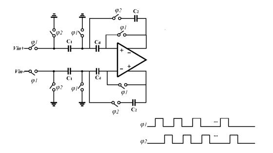
Fig. 3.7 CDS implementation in proposed ADC
