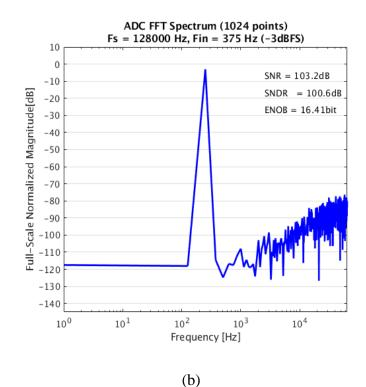
Fig. 3.8 (a) Simulated PSD without op-amp offset (b) with 5mV offset
