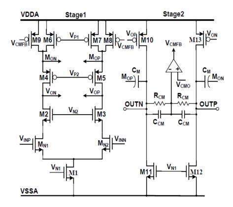
Fig. 2.13 Architecture of the op-amp used as integrator
