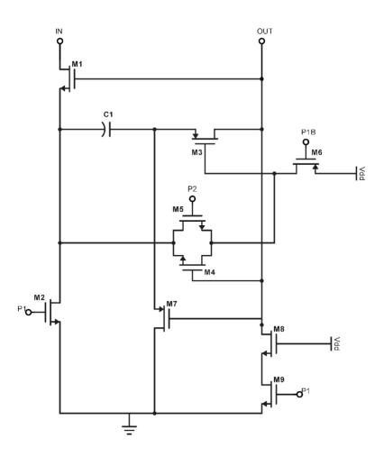
Fig. 2.17 Schematic of bootstrapped circuit
