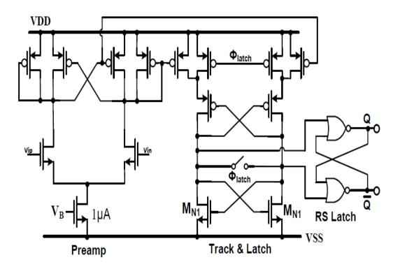
Fig. 2.14 Dynamic comparator used in proposed ADC
