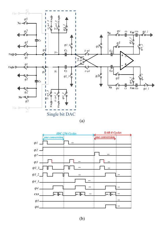
Fig. 3.20 IADC based calibration for the proposed NS SAR ADC
