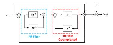
Fig. 2.7 Signal flow diagram of NS SAR with active integrator [4]
