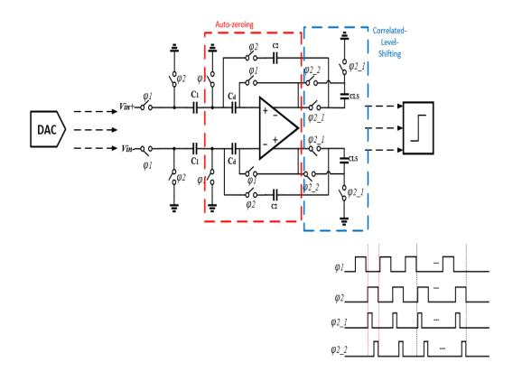
Fig. 3.13 Combination CDS and CLS to proposed NS SAR ADC
