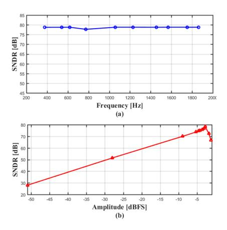
Fig. 2.20 (a) SNDR versus input frequency, (b) SNDR versus input amplitude
