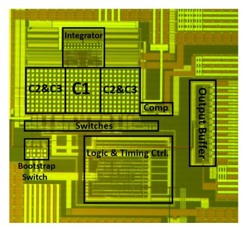
Fig. 2.18 Die photo of proposed NS SAR ADC
