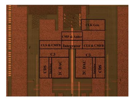
Fig. 3.29 Die photo of proposed NS SAR ADC
