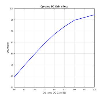
Fig. 2.12 Simulated SNDR versus op-amp DC gain
