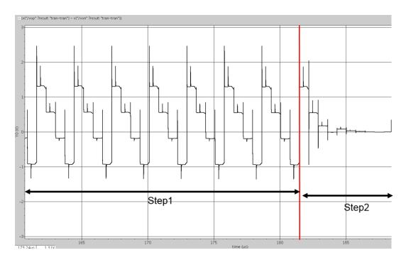
Fig. 3.23 Integrator output transient response in calibration mode
