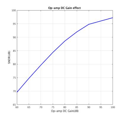
Fig. 3.9 Simulated op-amp finite DC gain effect
