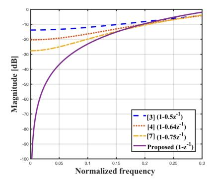
Fig. 2.11 Comparison of noise transfer functions
