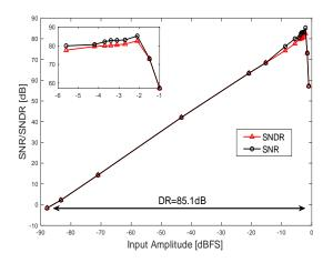
Fig. 3.32 SN(D)R versus input amplitude
