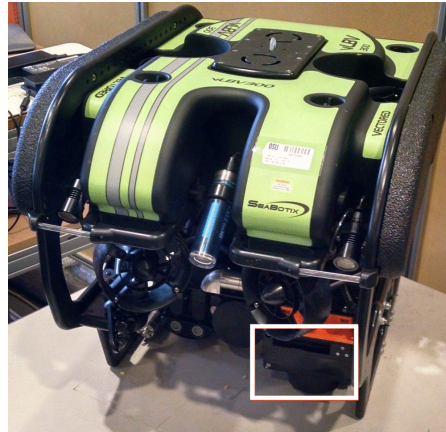
Figure 3.6: The Seabotix vLBV300 and Gemini 720i imaging sonar (designated by the white rectangle in the lower right).
