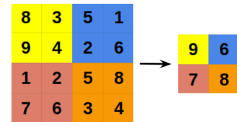
Figure 2.6: Max pooling using a 2D neighborhood
