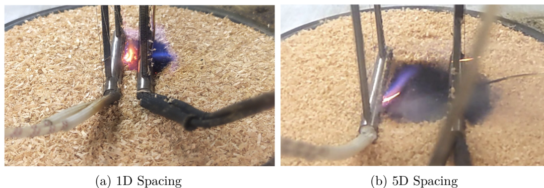
Figure 6.6: Images of fuel beds shortly after ignition near the upstream (left) heater. In both cases the wind speed was 5.8m/s and the upstream heater is unheated/inert. Air is travelling from left to right in both images.
