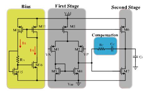
Fig 3.1: Low-Voltage PVT-insensitive tracking frequency compensated OTA
