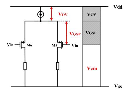
Fig 4.5: Common-mode input voltage range of PMOS input pairs
