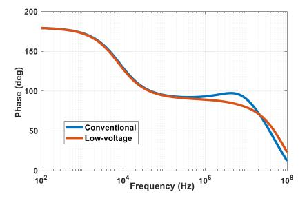
Fig 3.7: Comparison of the phase responses between conventional OTA and low-voltage OTA at  $V_{DD} = 1.4V$
