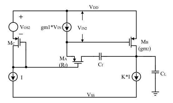
Figure 1.4: Tracking RC compensation
