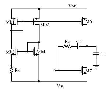
Figure 1.5: Method of relating  $g_{m7}$  with  $R_S$
