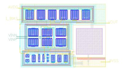
Fig 3.10: Layout of the conventional compensated OTA
