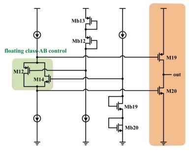
Fig 4.8: Output stage with floating class-AB control
