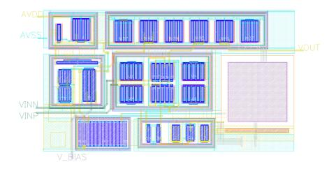
Fig 3.11: Layout of the low-voltage compensated OTA
