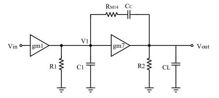
Fig 2.2: Block-level schematic of a Conventional PVT-insensitive tracking frequency compensated OTA
