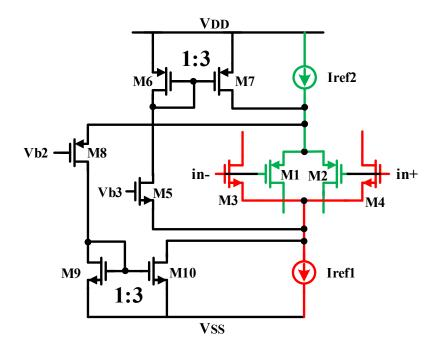
Fig 4.2:  $G_m$  control by current switches of rail-to-rail input stage
