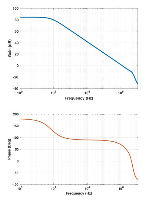
Fig 4.10: Loop gain bode plot of rail-to-rail operational amplifier
