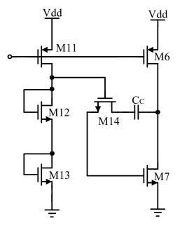
Fig 2.3: The bias circuit, second stage, and compensation network of the two-stage OTA
