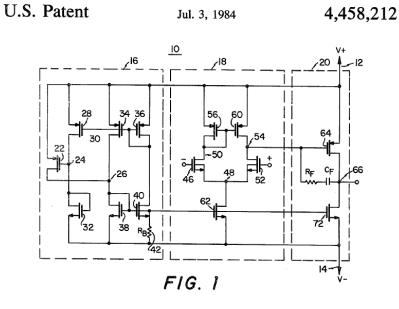
Fig 3.12: The two-stage compensated amplifier with pole-zero tracking [6]
