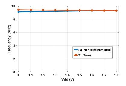
Fig 3.6: Non-dominant pole and zero frequencies of the low-voltage compensated OTA across different  $V_{DD}$
