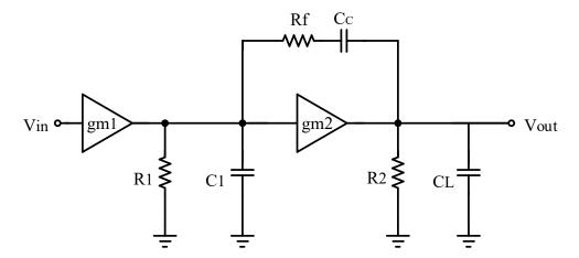
Figure 1.3: Small-signal model of RC compensation method
