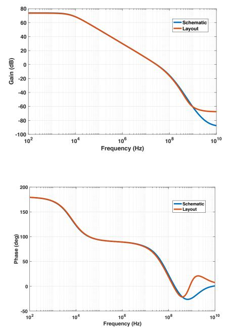
Fig 3.2: Loop gain bode plot of conventional OTA
