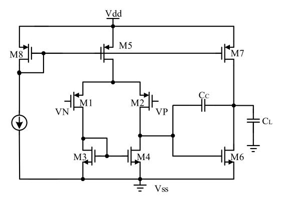
Figure 1.1: Conventional Miller compensated two-stage operational amplifier
