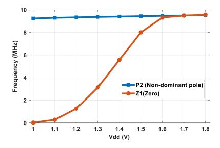
Fig 3.5: Non-dominant pole and zero frequencies of the conventional compensated OTA across different  $V_{DD}$
