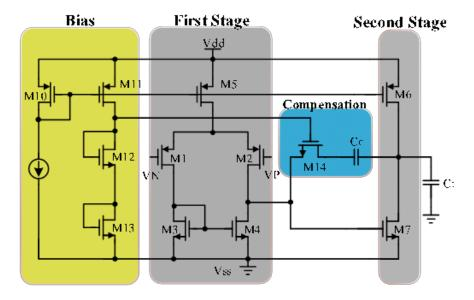
Fig 2.1: Conventional PVT-insensitive tracking frequency compensated OTA
