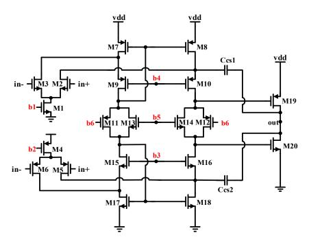
Fig 4.9: Cascode frequency compensation
