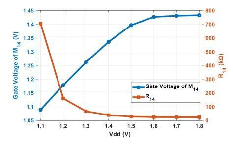
Fig 3.4: Relationship between gate voltage of  $M_{14}$  and its equivalent resistance,  $R_{14}$ , of the conventional OTA with respect to supply voltage.  $R_{14} = 24.2k\Omega$  at  $V_{DD} = 1.8V$
