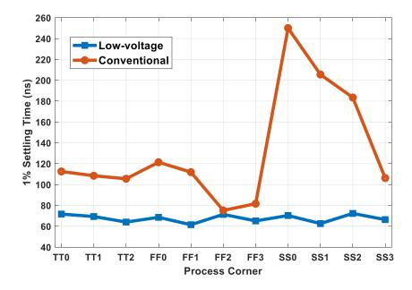
Fig 3.9: 1% settling time comparisons between the conventional and low-voltage compensated OTA
