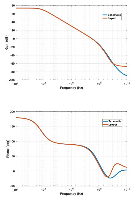
Fig 3.3: Loop gain bode plot of low-voltage OTA
