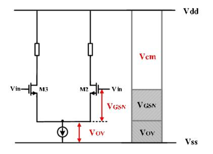
Fig 4.6: Common-mode input voltage range of NMOS input pairs
