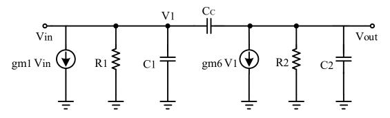
Figure 1.2: Small-signal model of conventional Miller compensated OTA
