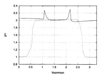
Fig 4.1: Normalized transconductance,  $g_m$ , across common mode input voltage [15]
