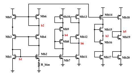
Fig 4.4: Bias circuit of rail-to-rail amplifier
