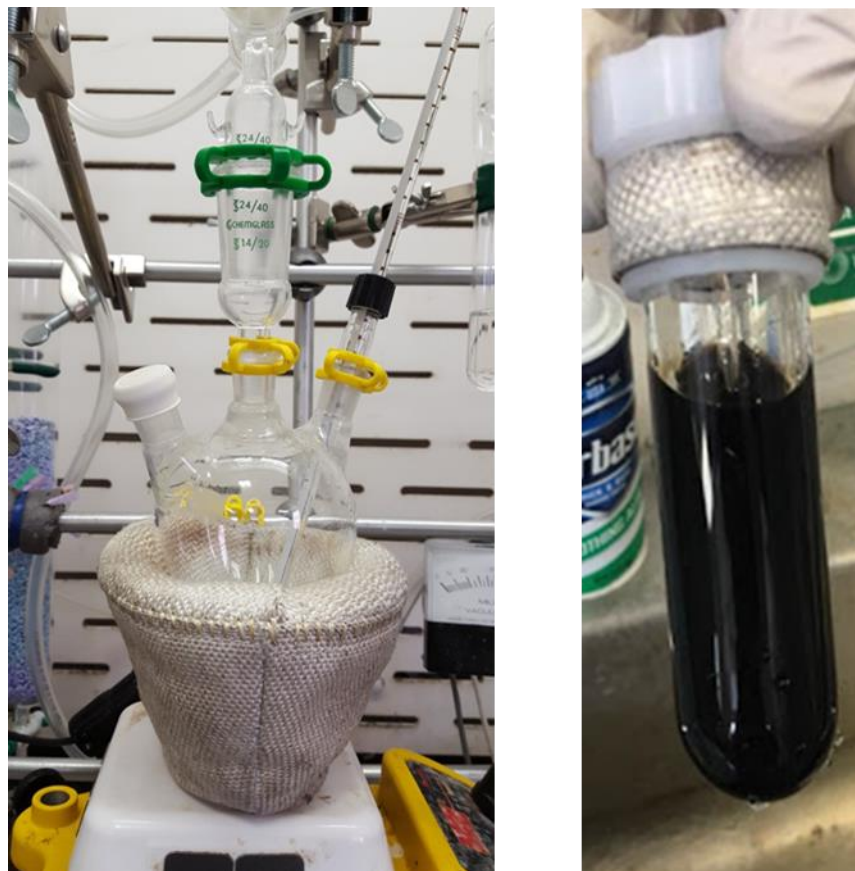
Fig 32. a) Precursor dissolution setup w/ heating jacket. b) The reacted precursors, post-microwave step turns into a black colored solution indicating reaction completion to form PbSe NC.
