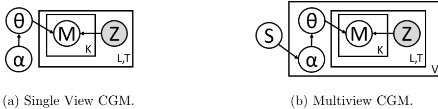
Figure 4.2: Plate diagrams for single view and multiview CGM. K represents the neighborhood size of the graph, V the number of data views, L the number of locations and T the number of time steps.
