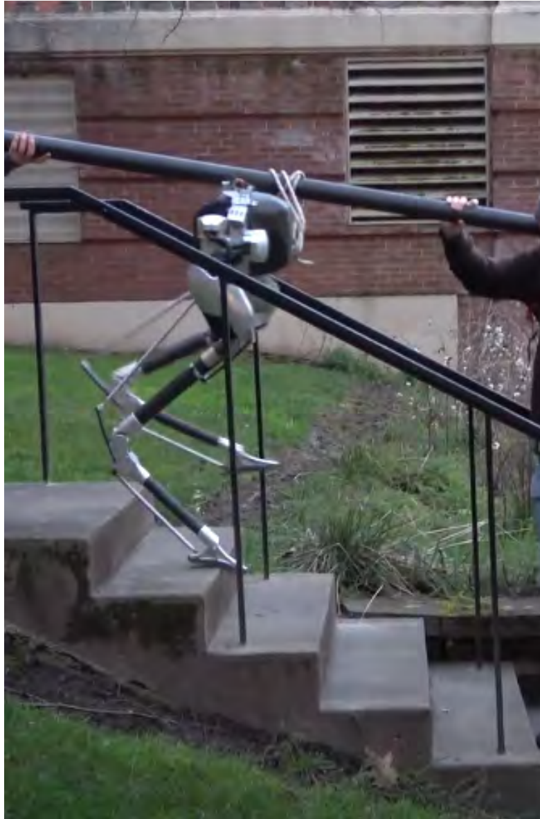
Figure 4.4: The learned policies exhibit a high degree of blind robustness to a variety of stair-like terrain, and can reliably ascend and descend stairs of typical dimensions found in human environments.
