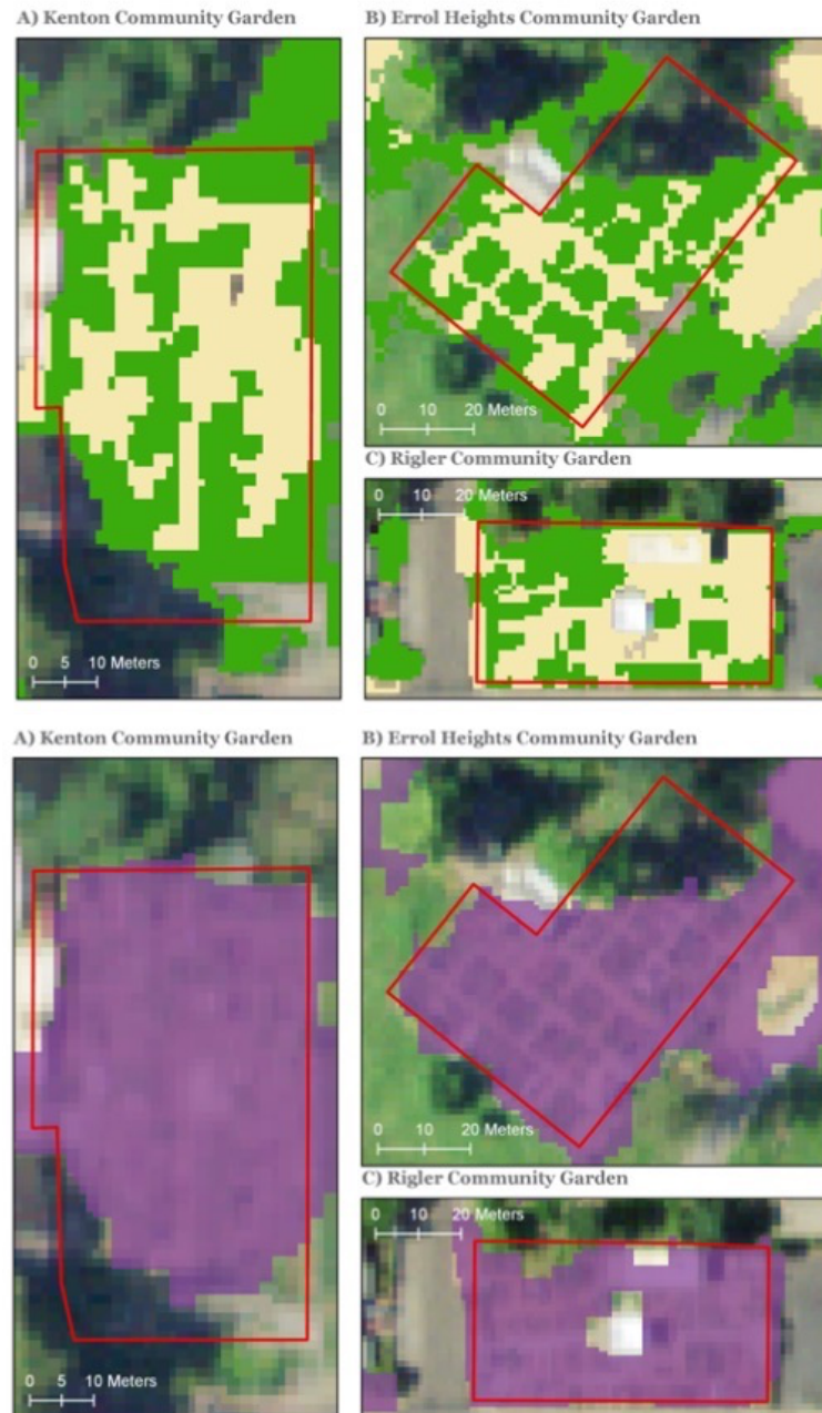
Figure 2.13. Sample garden 1) classes (garden vegetation in green and bare in yellow) and 2) garden pixels (purple). A) Kenton Community Garden is almost completely covered by the two classes other than the shaded area in the southwest corner. With an 80% detection rate, the same area appears in the garden pixels, with the exception of the northeast corner which is consistently vegetation. B) Errol Heights Community Garden follows a similar pattern with the two classes other than the shaded area in the northern corner, with matching garden pixels with 77.8% detected. C) Rigler Community Garden has the two classes throughout the garden other than the structure in the middle of the garden and along the north side. The garden pixels mirror the garden classes detecting 86.3% of the garden.
