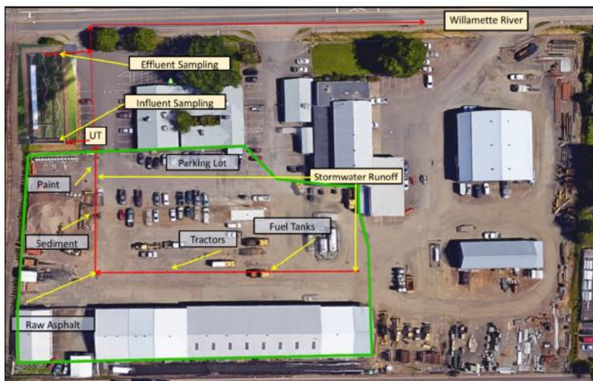
Figure 3.1 Aerial view of the OGSIR facility and the Benton County Public Works transportation yard. The catchment is outlined in green, the runoff paths are shown in yellow, and the pre-existing city storm drainpipes are shown in red (Source: Kshitiz, 2018).
