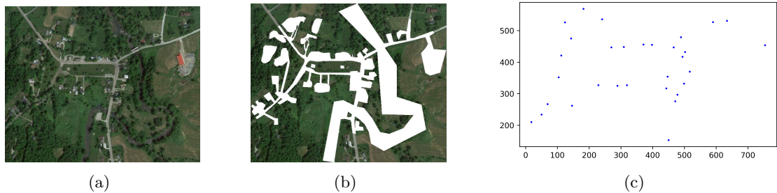
Figure 2.4: (a) Google Earth U.S. town image, (b) with exclusion zones, such as houses and roads and rivers, highlighted in white, (c) house locations as located on the image
