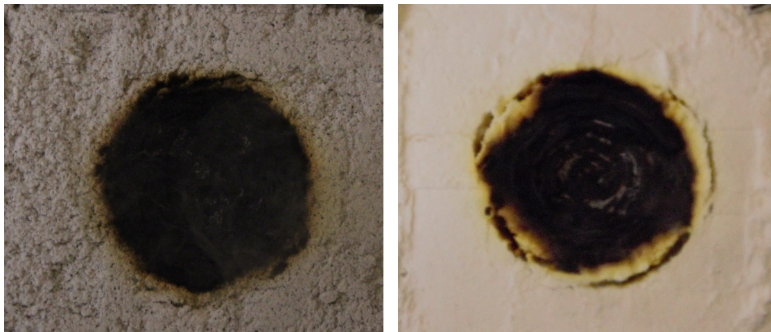
Figure A.14: Images for burns with 100% cellulose (right) and 80% cellulose/20%lignin (left). Numerous large, dark cracks are visible outside the burned area in the 100% cellulose case.
