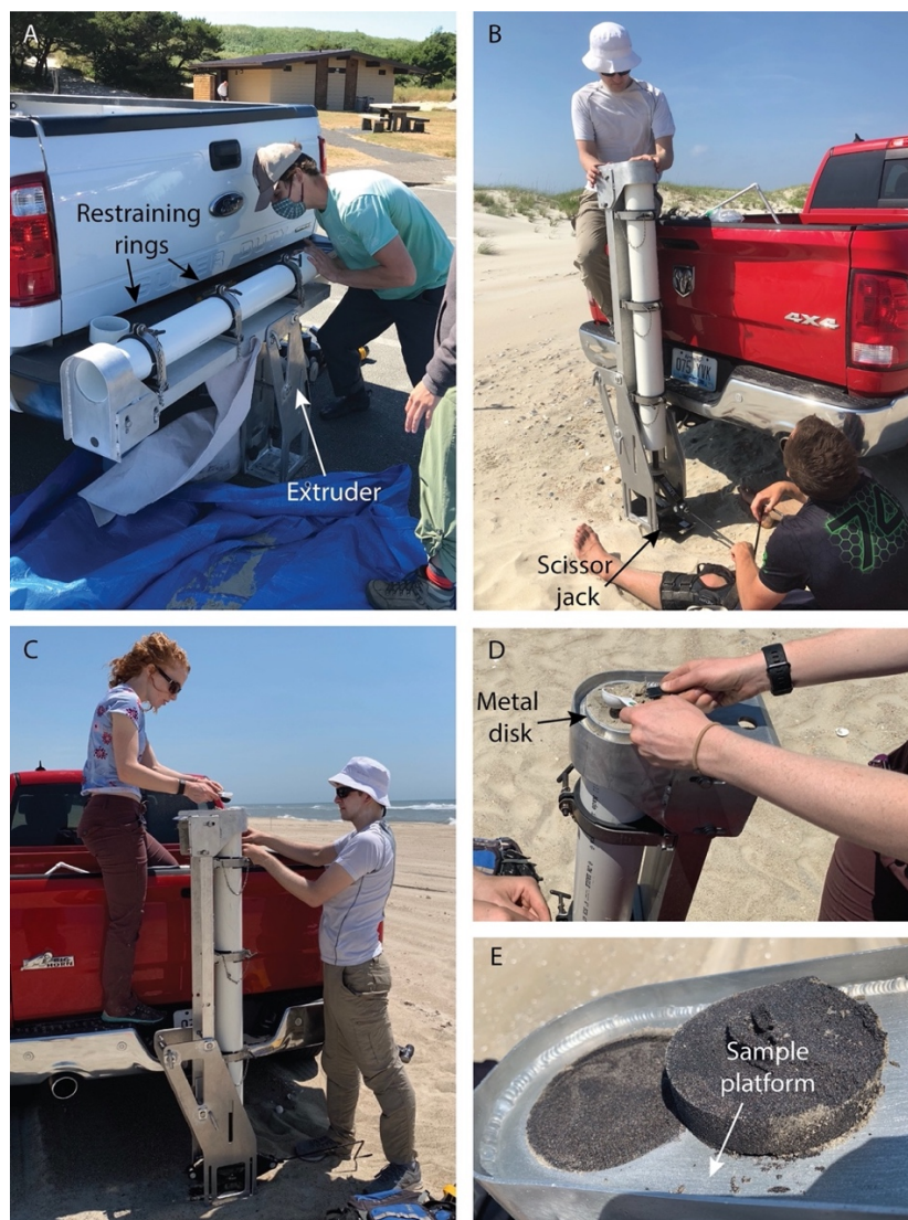
Figure D3. Methods and equipment for extruding sand sediment from dune cores. (A) Following core collection, the custom-built extruder (Figure D2) was attached to the truck hitch and the core tube was loaded into the extruder in the horizontal position so that the four restraining rings could be tightened around the core tube (see Figure D2a). The test plug was then removed from the top of the core (with the plastic end cap still in place) before fastening the extruder in the vertical position for use (Figure D2b). (B) During use, the extruder was stabilized from above by one person while another person used a scissor jack to insert the spacers into the core tube and slowly extrude sediment from the top. (C) and (D) A 2-cm high metal disk (10-cm diameter) was placed at the top of the core to extrude sediment in 2-cm increments for sampling. A tablespoon was used to scoop samples from within the 2-cm sample disk. The remainder of the sample was discarded, and the metal disk and sample platform were cleaned with a brush. (E) Samples were collected every other 2-cm increment and the samples in between those increments were discarded.
