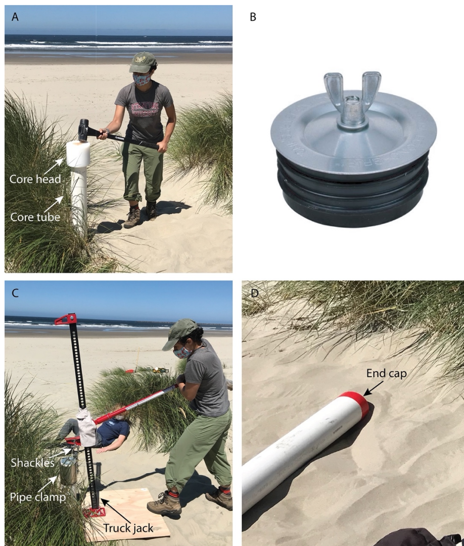
Figure D1. Methods and equipment used to collect sediment cores in dunes. (A) Core tubes (10-cm diameter PVC pipe) were pounded into the toe, crest, and heel of the foredune using a sledgehammer and custom ‘core head’ placed over the top of the core tube to provide a surface for pounding. (B) Once the core tube was pounded into the dune, a test plug was inserted within the tube (above the sediment) to prevent sediment loss upon removal. (C) A pipe clamp and shackles were used to attach the core tube to a truck jack (attached to a plywood board) in order to remove the core from the dune. At times, the truck jack became too clogged with sand to use; in such cases, the cores were dug out of the dune using shovels. (D) A plastic end cap was placed over the end of the core tube upon removal to prevent any sediment loss. Core tubes were transported upright to avoid disturbing layers within the core.
