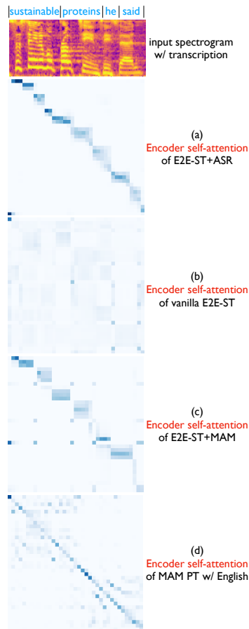
Figure 4.8: One head of the last layer self-attention comparison between different models. ASR MTL and MAM help the encoder learns similar self-attentions.
