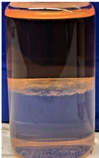
Figure 4-8. Contacting effluent from SAP waste with 30% TBP in TCE resulted in third-phase formation at the aqueous-organic interface
