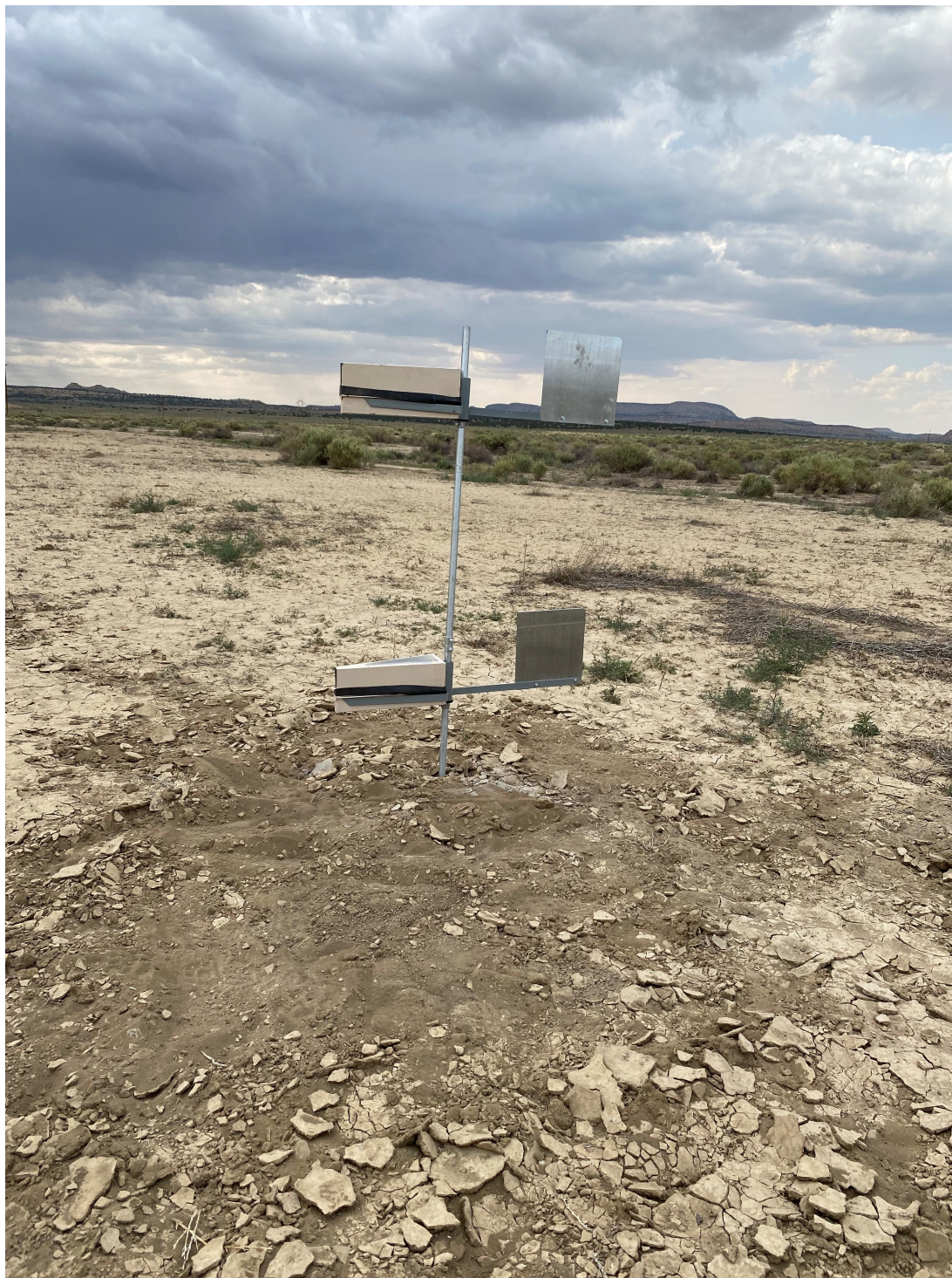
Figure 3.1: BSNE sampler setup at the unremediated section site
