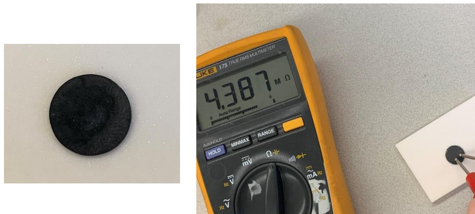
Figure 6.4: Images of (a) synthesized and polished dense BFN-1 ceramic showing dark metallic appearance, and (b) resistivity measurement of as-polished surface with a laboratory voltmeter of the dense BFN-1 ceramic
