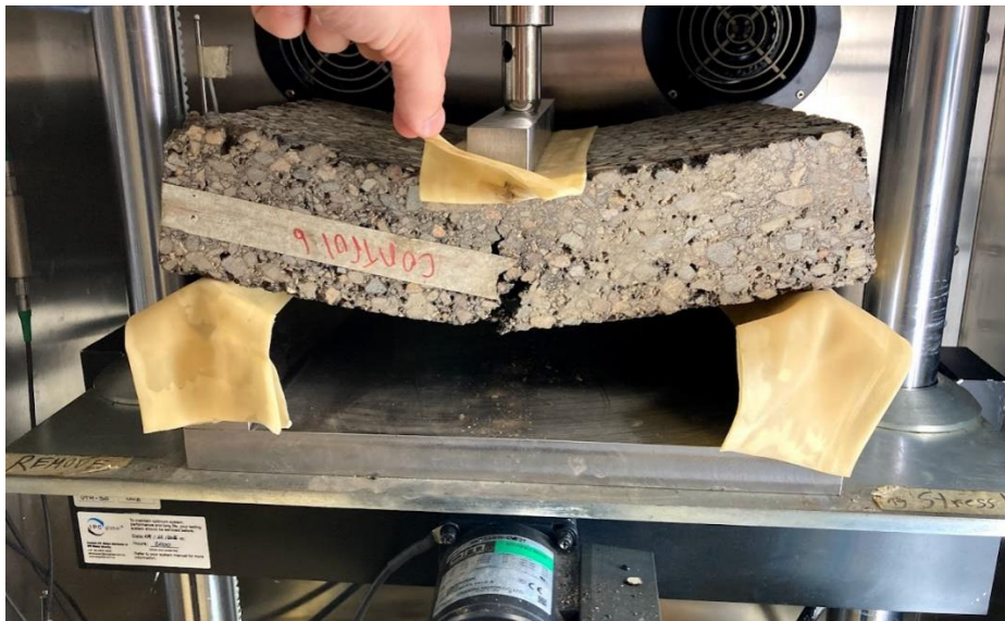
Figure 4.10: Tested three-point flexural fatigue sample
