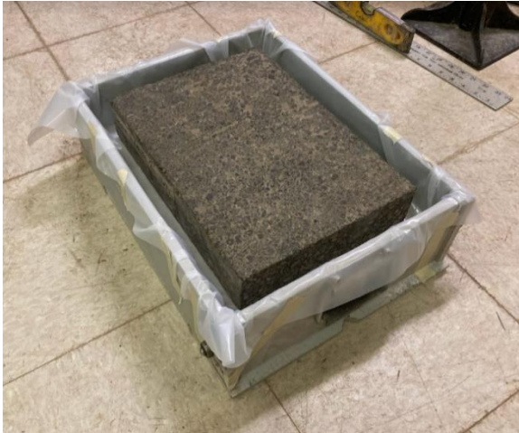
(c) Asphalt sample centered in HWTT mold
