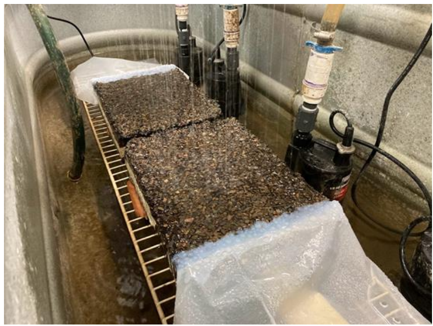
(b) Sample undergoing infiltration test
