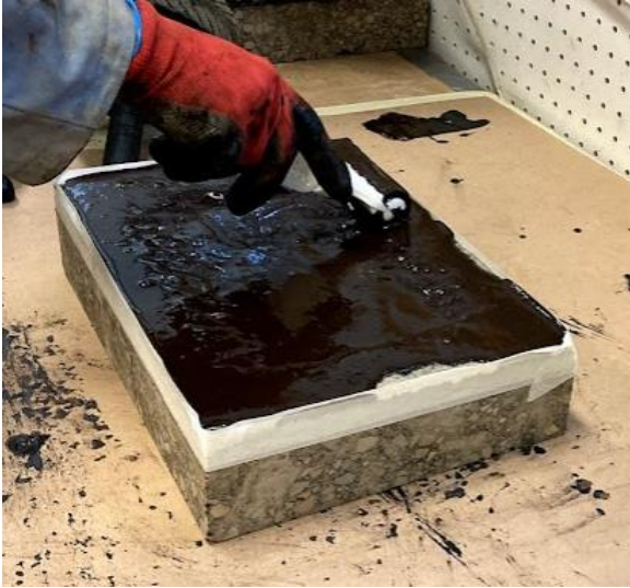
(c) Spreading emulsion
