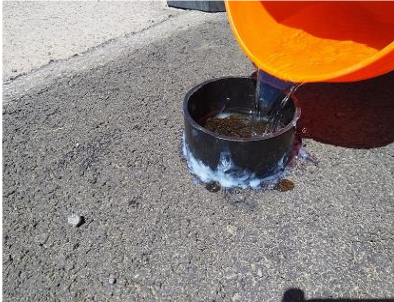
Figure 4.4: Field infiltration test
