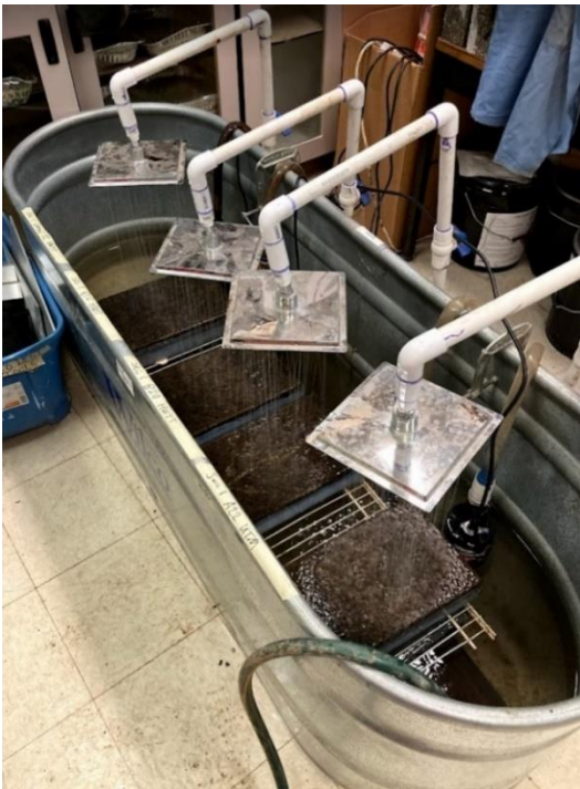
(c) Sealed samples undergoing rainfall simulation
