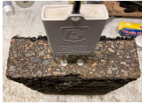
(b) Sand and sensor inserted
