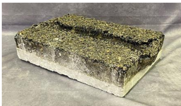
(b) Control, Freeze-Thaw & Chip Seal
