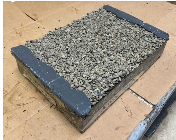
(d) Devcon used to flatten ends due to chip seal aggregates
