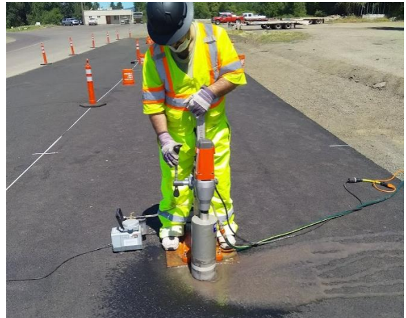
(f) Coring for lab density measurement and testing
