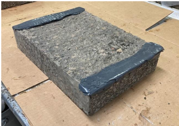
(c) Devcon used to flatten ends due to rumble strip curvature
