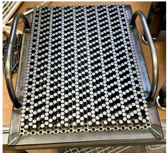
(b) Aggregate restrainer with specialized bolt layout
