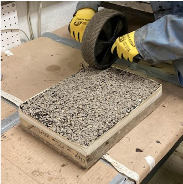
(e) Compacting aggregates
