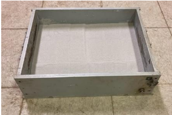
(a) HWTT mold with sand base layer
