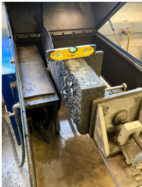
Figure 4.8: Cutting samples using water-cooled diamond blade
