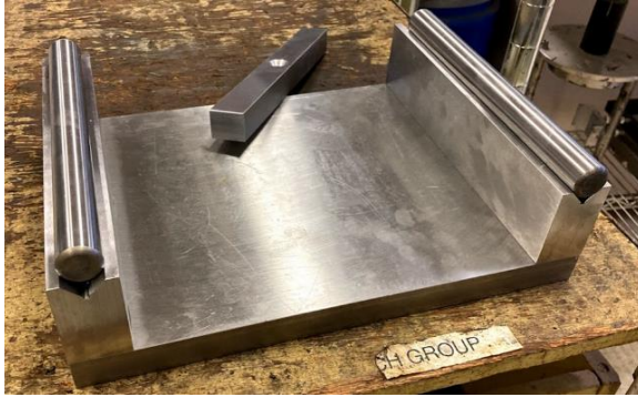
(a) Three-point bending frame
