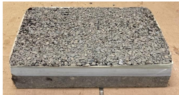
(f) Finished CLRS chip seal block sample
