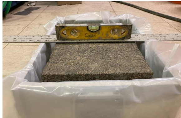
(b) Asphalt sample level with the surface of HWTT mold
