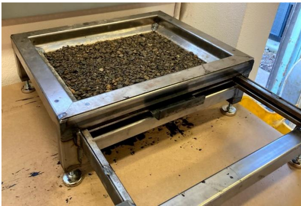
(a) Aggregates spread evenly atop spreader sheet
