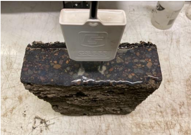
(c) Moisture sensor sealed with silicone gel
