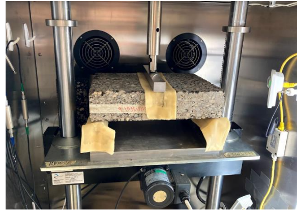
(b) Three-point bending sample positioned in the Universal Testing Machine (UTM)
