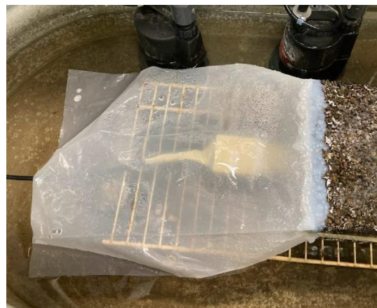
(e) Protective covering placed over sensor area
