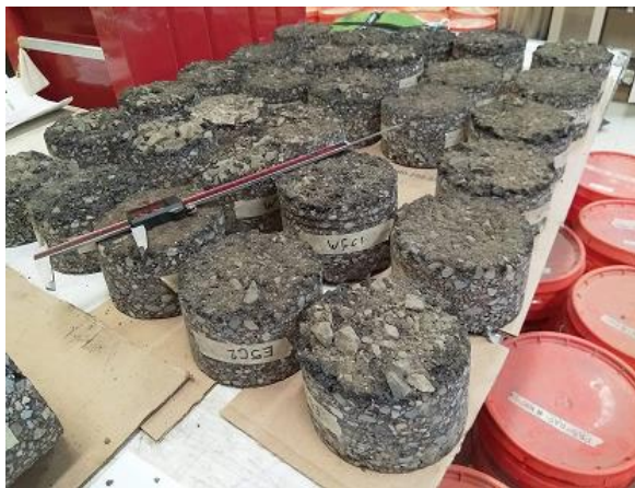
(g) Sampled asphalt cores
