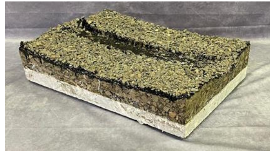
(f) Sinusoidal, Chip Seal
