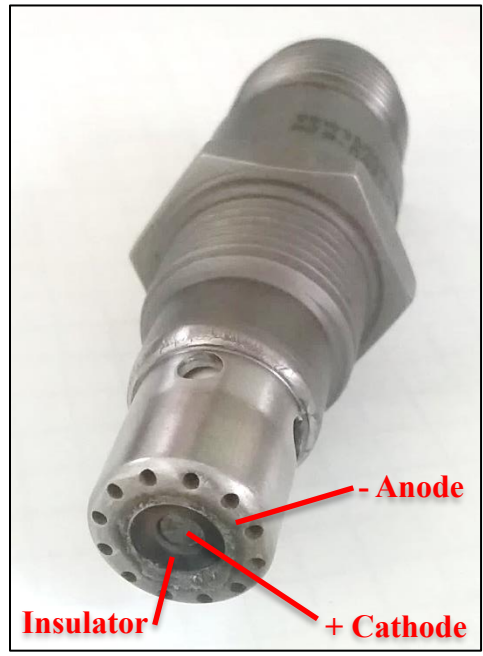
Figure 6 Photograph of the igniter used in this work.
