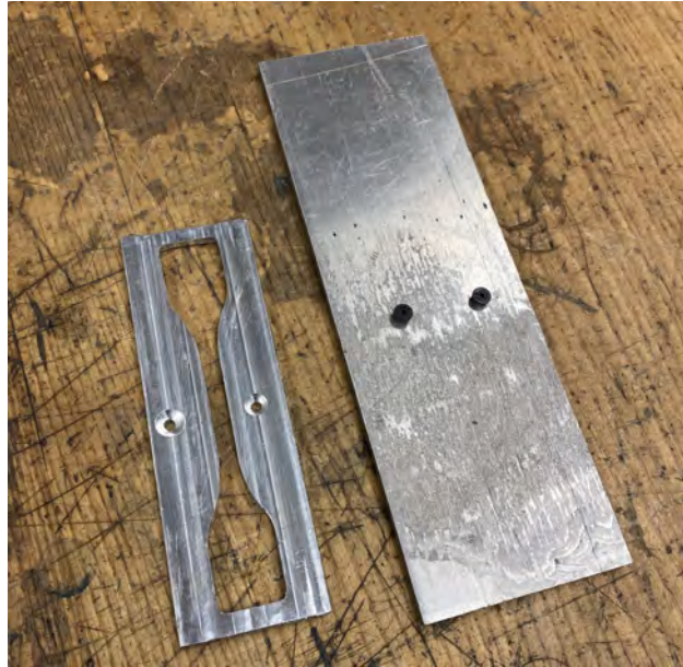
Figure 6: Two part aluminum mold for heat pressing.
