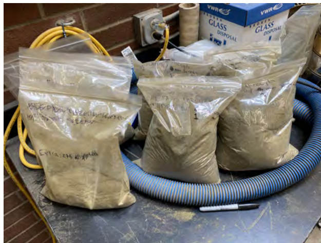
Figure 2: Hemp particles sorted by size after the grinding and sieving process.
