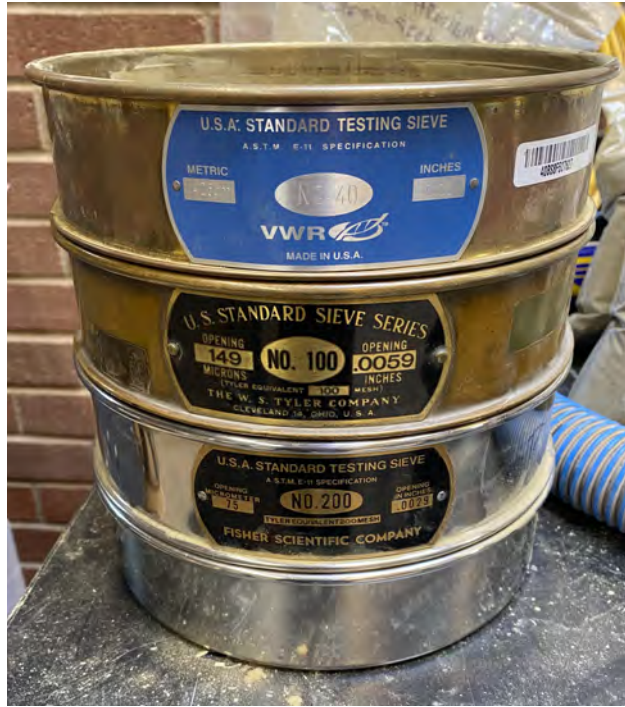
Figure 1: Sieves used to filter hemp particles to 75-149 micrometers.
