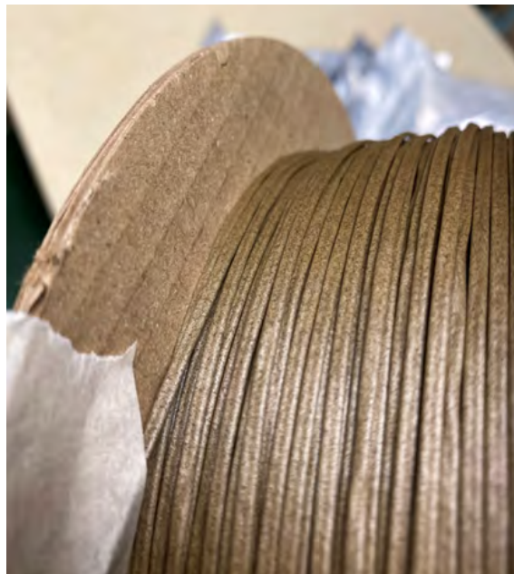
Figure D.4: Collapsed 15 wt% Protopasta custom filament
