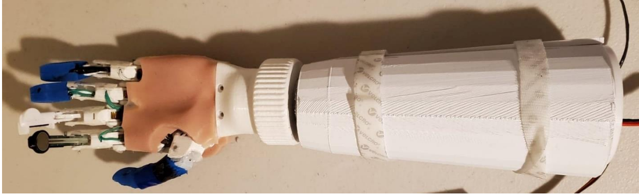
Figure 2: Testing set-up where the index finger has an FSR on the end.
