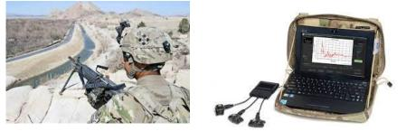
(Left) Blast Gauge Field Testing-Afghanistan, 2014. [112] (Right) Blast Gauge System. [113]
