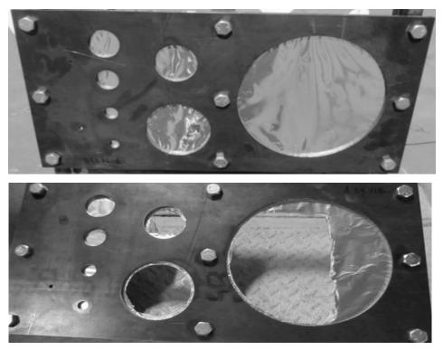
Cold War-era shockwave gauges, named "Bikini Gauges" after the Bikini Atoll, intact (*top*) and after blast exposure (*bottom*). [109]
