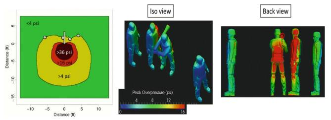
Diagram displaying blast overpressure impulse levels from an M-48 Carl Gustav Recoilless Rifle.[87]
