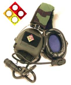
Shockwave Exposure Indicator prototype affixed to hearing protection.
