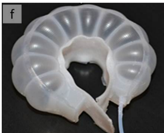
Figure 2: The figure is an example of a silicone pneunet fully bent [13].
