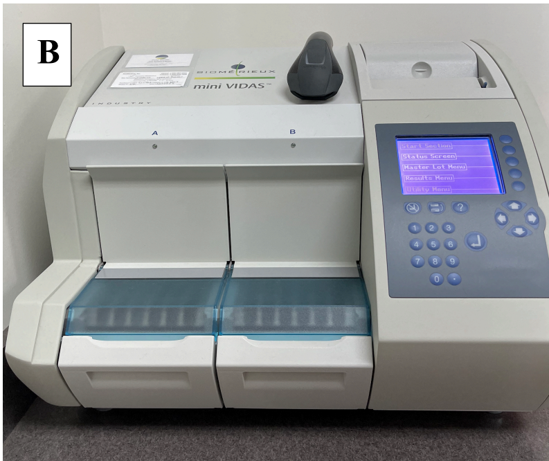
Figure 1: The CIA progesterone analyzer (A) and ELFA progesterone analyzer (B) used in this research.
