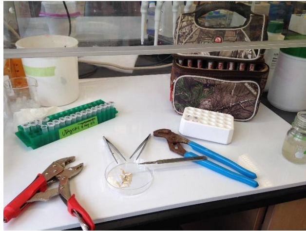
Figure 3: Photo of the filter cracking and cutting process (Dawn Urycki)
