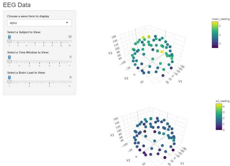
Figure 4: The app used for exploratory analysis. The slider bars on the left allow the user to filter through the different subjects, time windows, and brain loadings. The top graph shows mean readings for each sensor node under the appropriate filters, whereas the bottom graph shows the standard deviation of each node reading under the appropriate filters.
