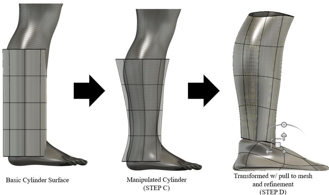
Figure 14: Above is a series of screenshots that show the shaping process that takes place during surface modeling. This series is from the prosthetic casing for Connor, but a similar approach was taken when designing the casing for Rio.
