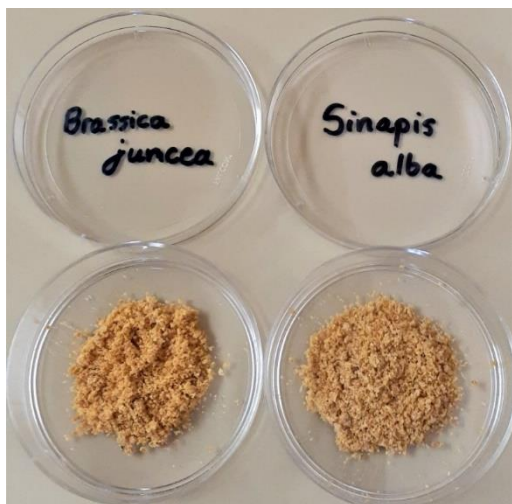
Figure 3.2. Image of Brassica-origin seed meal in powdered form indicated lack of requirement for the extraction protocol and need for standardized leeching process. This also shows comparison in the composition of the two different substances, where the B. juncea is clumpier and likely contains more moisture than S. alba .
