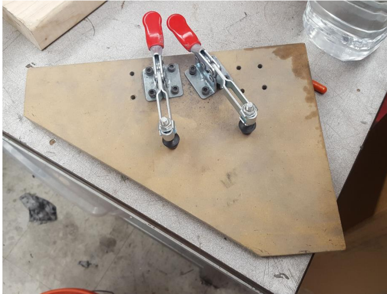
Figure 8: Fin bevel fixture.
