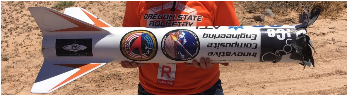
Figure 16: Lower airframe and fins post competition launch
