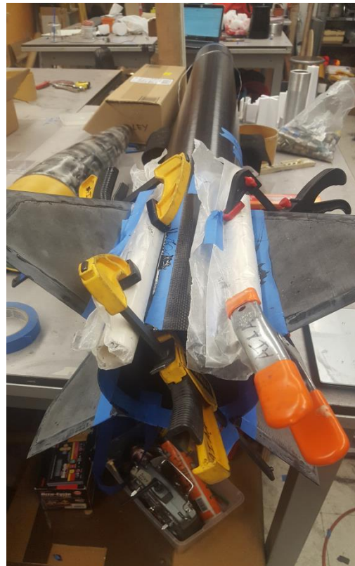
Figure 11: ½” epoxy fillet setup.
