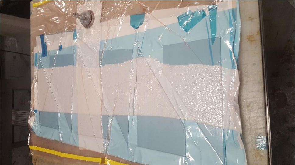
Figure 7: Vacuum bagged fins.
