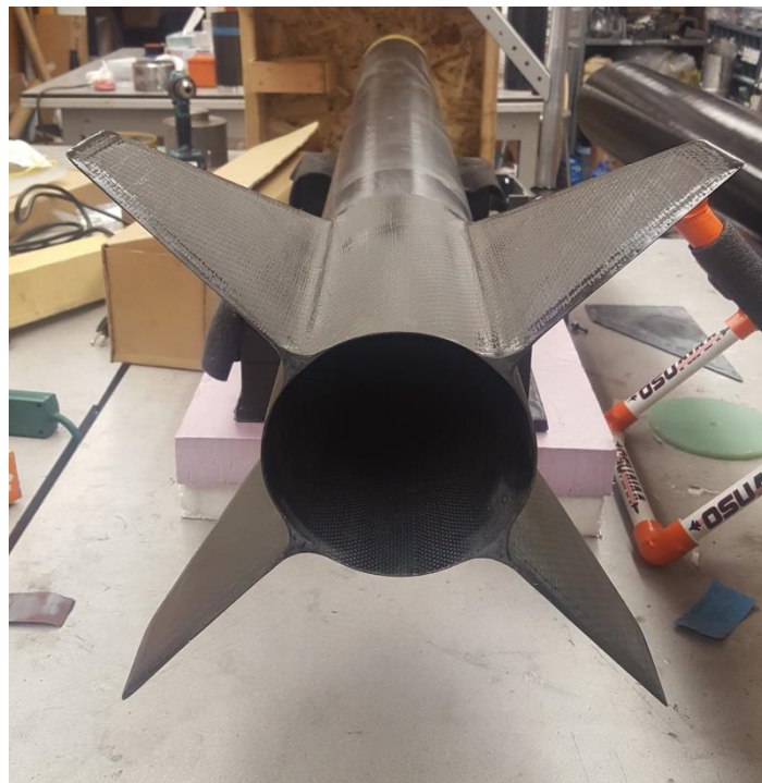
Figure 13: Completed tip-to-tip layup
