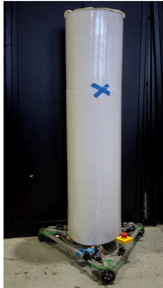
Figure 3.4: The robot has a simple body with an X marking the front, an omnidirectional platform, and a maximum speed of 1.5m/s
