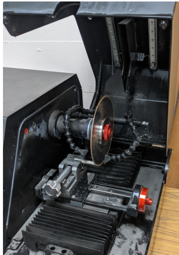
Figure 3.1.2 Process of cutting disks from the billet inside a diamond saw
