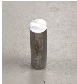
Figure 3.1.1 Machining billets from the as-received material
