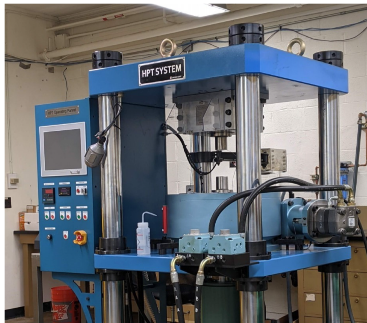
Figure 3.1 HPT System in the Advanced Materials Processing and Analysis Laboratory
