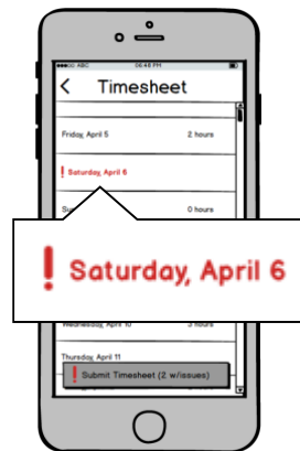
Fig. 7. The potential fix from Team 1A, with UXpert feedback, for Bug #4. Displays the remaining days as a list, with red ‘!’ notifications and text for days with problems.
