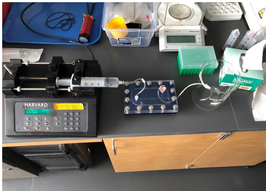
Figure 16 – Syringe pump set-up during a cleaning procedure before actual flow of blood using isopropanol and water.
