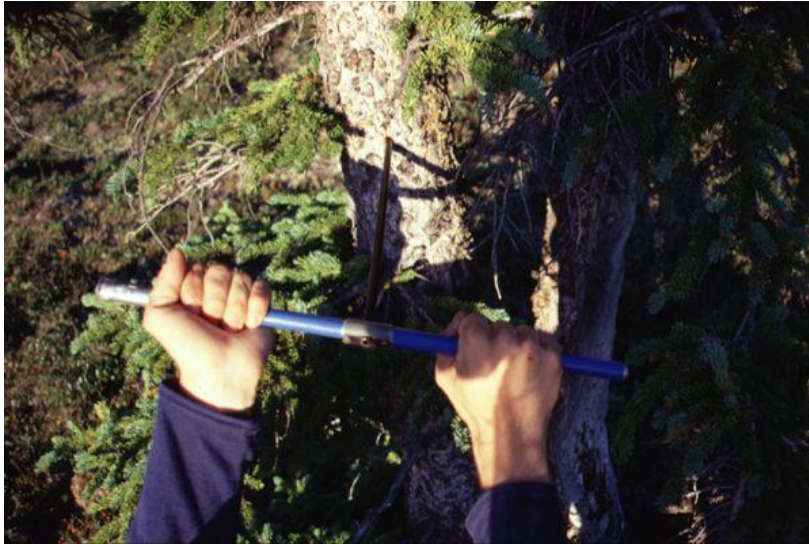
Figure 6. Incremental borer used to determine age and growth of a tree
