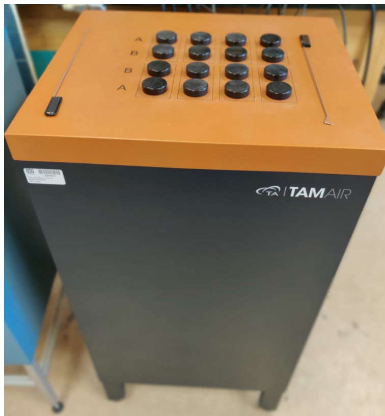
337 Figure 4-5. TAM Air isothermal Calorimeter used for heat flow measurements from 338 samples
