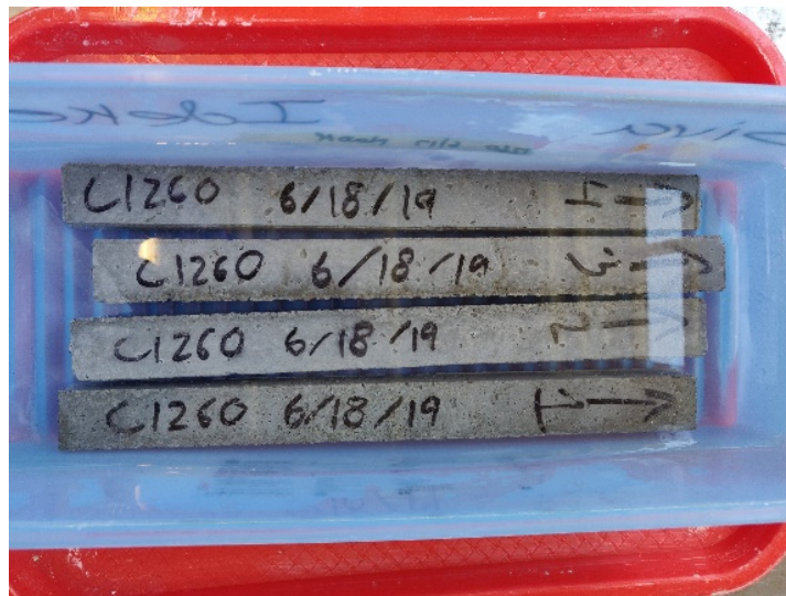
664 Figure 5-11. ASTM C1260 mortar bars immersed in 1N NaOH solution in a test container; 665 note that the length of each prism is 285 mm for scale.
