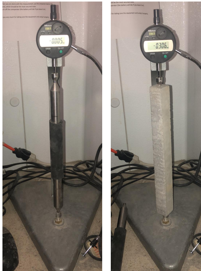
991 Figure 6-5. Drying shrinkage Comparator where a) illustrates the reference bar's 992 measurement and b) shows the sample's measurement.
