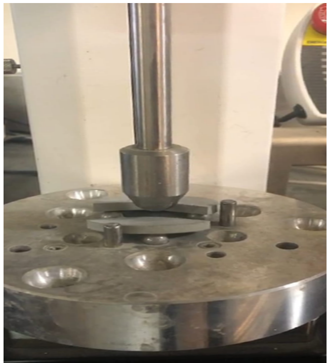
1133 Figure 7-1. The Experimental Setup for the B3B test: a) without the sample b) showing a 1134 mortar disk during testing and c) showing a mortar disk after testing (note the three 1135 vertical pins provide no restraint and are only used to locate the sample)
