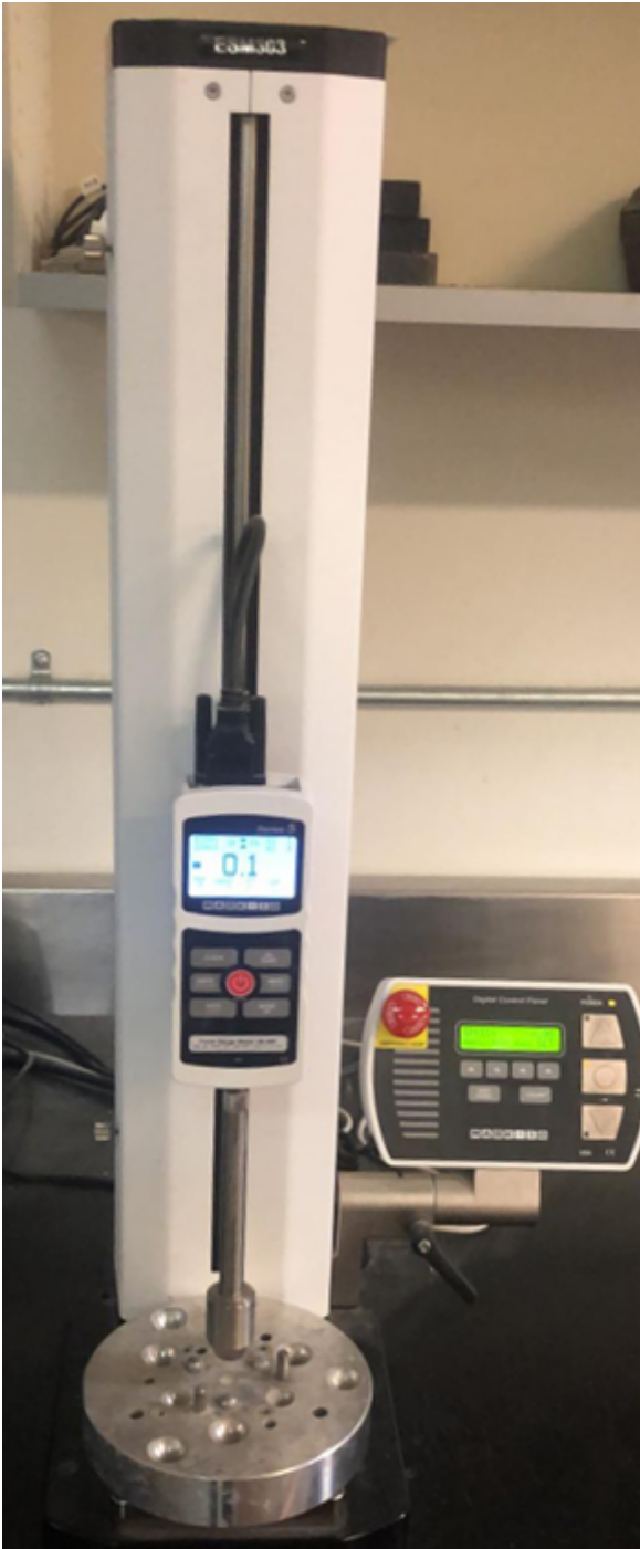
1133 Figure 7-1. The Experimental Setup for the B3B test: a) without the sample b) showing a 1134 mortar disk during testing and c) showing a mortar disk after testing (note the three 1135 vertical pins provide no restraint and are only used to locate the sample)
