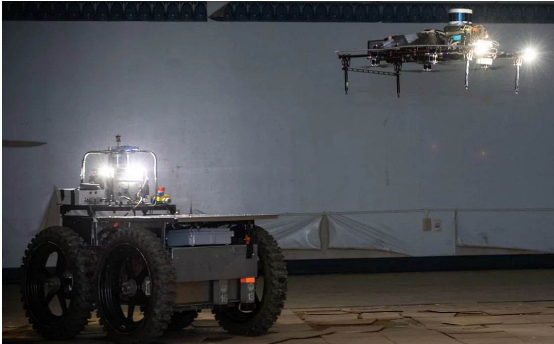
Figure 1.1: An example of a marsupial robot system by Team Explorer (CMU and OSU) [1]. The carrier robot on the left has increased payload capacity, better sensor capabilities, and longer battery life. The aerial passenger robot on the right is more lightweight and has better agility compared to the carrier robot.
