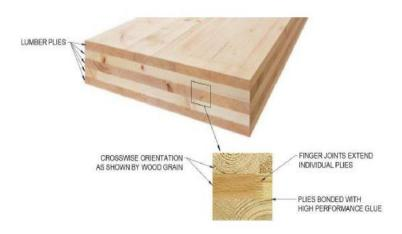
Figure 2. 1 Schematic of CLT panel (Kordziel, 2018)
