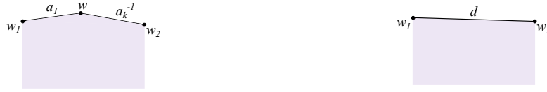
Figure 8.7: Replacing the edges a_1 and a_k^{-1} with a boundary dummy edge d .
