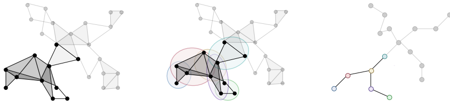
Figure 4.1: A subtree rooted at t and the corresponding subcomplex K_t . Notice that the triangle is excluded from the topmost bag X_t .
